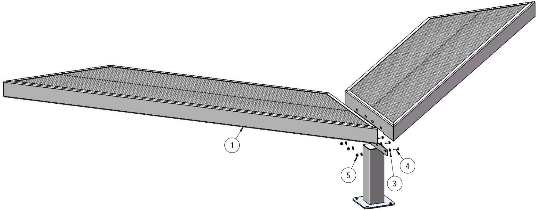
Attach two of the 8' benches to a 934 Leg using specified hardware as shown. Repeat this using the other two benches.
