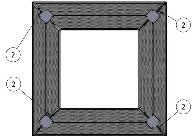
Attach the two halves of the square together using the other two legs and hardware.
