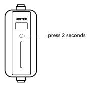
Please press the button for 2s to enter adjustment mode, with [CUR] and [APPT] are optional, respectively for adjusting the charging current and setting the charging appointment time. Shortly press the button to switch options, Press 2s the button to enter the corresponding setting option.
