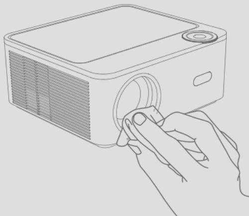
Gently wipe the lens by a piece of moistened (with a little water), non-abrasive and lint-free cloth to remove stubborn dirt.
