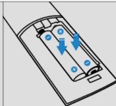
2. Insert batteries with the + and – ends as the indicators on the battery box showed;
