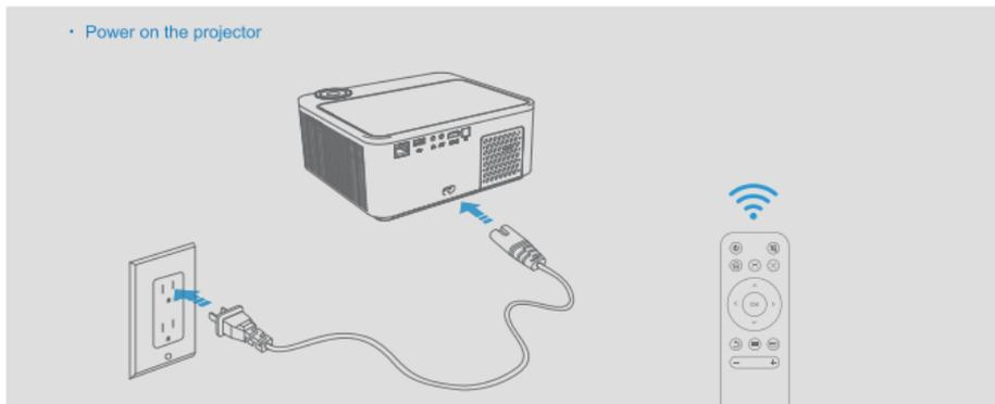
Indicator light will on after plugging in the power cord. Then press the Power button on the projector or on the remote control, it enters into multimedia interface within 2 to 5 seconds.
