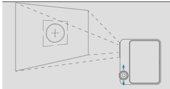
Rotate the focus ring to adjust the clarity of the projected image until it reaches to crystal clear.
