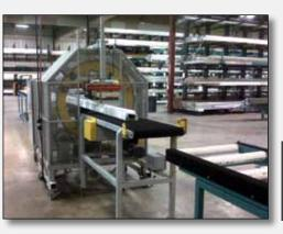
Industrial wrapping machines and heavy cardboard endcaps protect your panels from damage.
