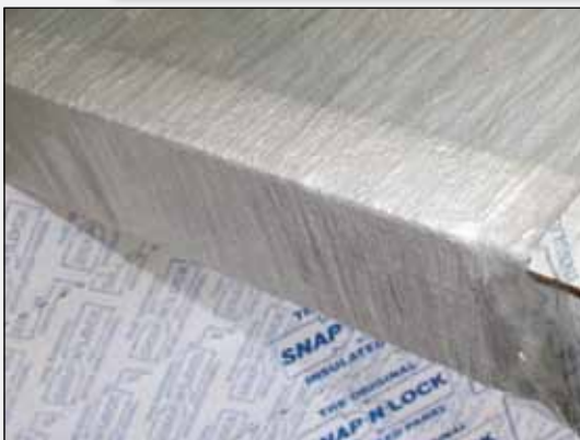
▲ Foam bumpers are used on both the male and female sides of the panels to prevent accidental denting and scratching.
