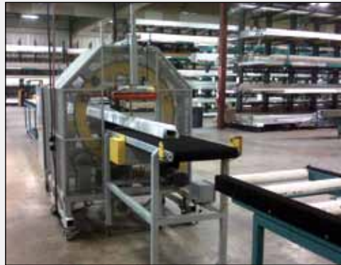
◀ Industrial wrapping machines and heavy cardboard endcaps protect your panels from damage.
