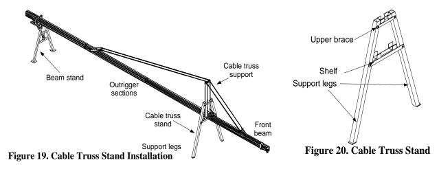
The Cable Truss Stand (see Figure 19) is designed to support the base of the 8 ft. Reach Cable Truss. Note that the standard Beam Stand (WS BS 001) must not be used to support the Cable Truss System. The Beam Stand is used to support the rear of the Cable Truss System. The Cable Truss Stand must be installed prior to the installation of the Cable Truss System. The installation procedure for the Cable Truss System with the Cable Truss Stand is as follows:
