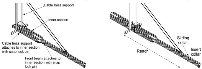
Figure 17. Front Beam - Inner Section - Cable Truss Support Assembly
