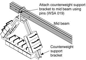
Figure 28. Counterweight Support Bracket Installation
