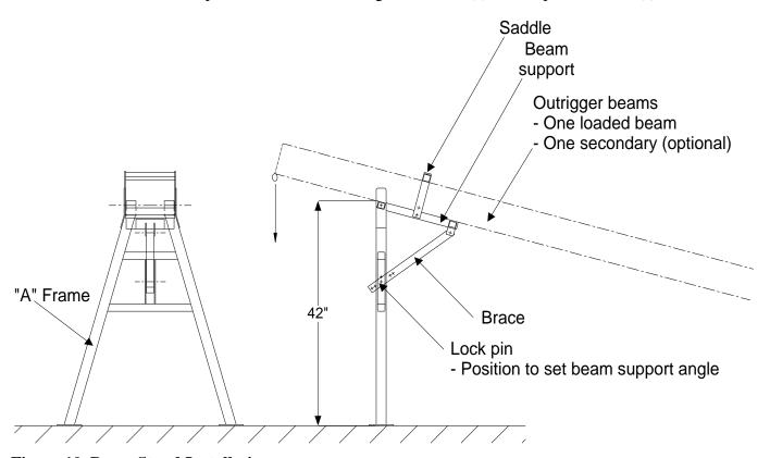
Figure 10. Beam Stand Installation
