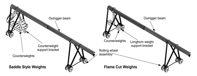
Figure 24. Rolling Outrigger
