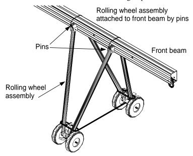
Figure 27. Rolling Wheel Assembly with Front Beam
