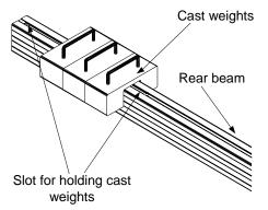
Figure 2. Rear Beam Holding Cast Weights
