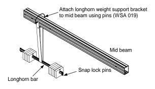
Figure 29.Longhorn Weight Support Bracket Installation
