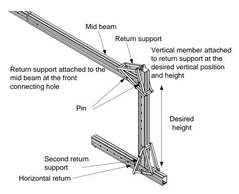
Figure 22. Return Support – Mid Beam Assembly
