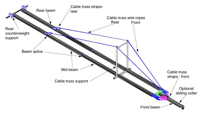
7. When moving the Cable Truss System into position ensure that the support for the front of the beam is located directly beneath the support feet of the Cable Truss Support. Do not support the Cable Truss System on either side of the Cable Truss Support as this places the load on the aluminum beam and not on the Cable Truss Support and can damage the aluminum beam.
