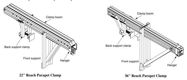
Figure 30. Parapet Clamp
