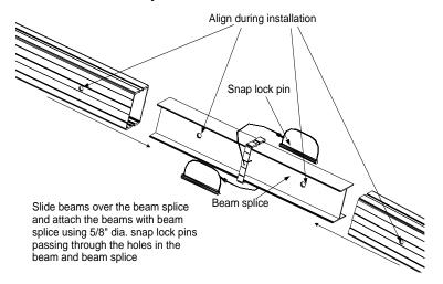
Figure 7. Assembling Beams with Beam Splice
