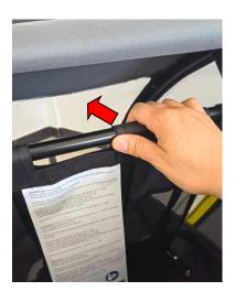
**Step 22:** Pull the horizontal rear tube forward.
