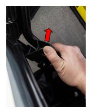
**Step 3:**Lock the buckles on both sides (2 with blue lever for locking and 2 without for reinforcement). The blue lever will be fixed and set automatically into position.
