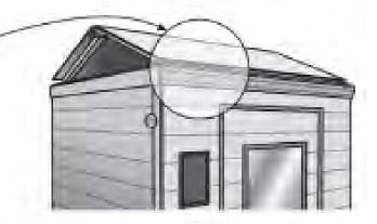
Next, take the clear plastic lining and cover the roof peak completely prior to installing the canvas cover.
