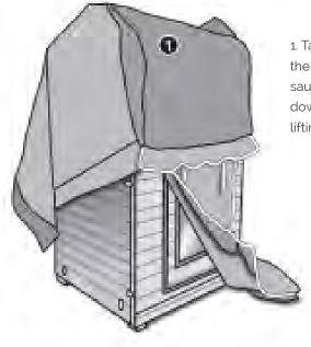
1. Take the back section of the cover and put it over the sauna. Pull the cover slowly down from the back while lifting up the front section.
