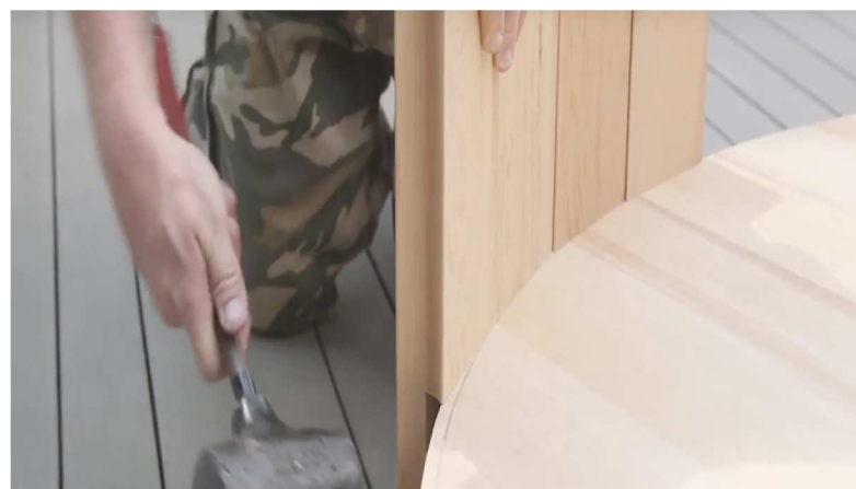
11. Use rubber mallet to ensure snug fit.
