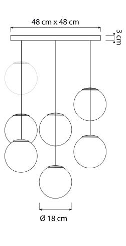
Sei lune ( 6 x Ø 18) max 6 x 8W | E14 (230V) - E12 (120V) Equivalent W dimmable LED bulbs compatible | rec. LED 6 x 3,5W
