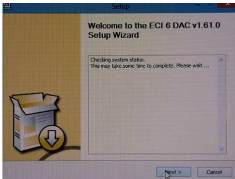
3. Press Next, then confirm or change the folder for the installation. Press Install when done.
