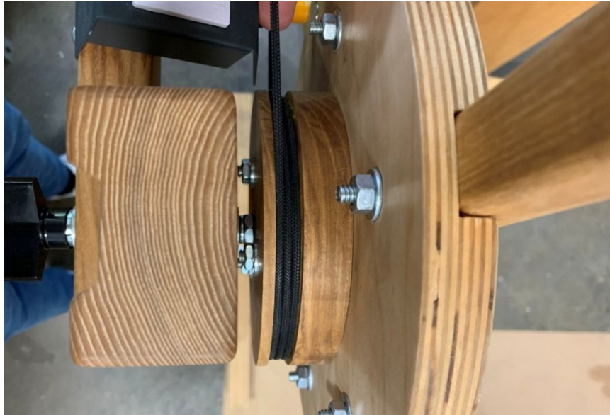
Figure 7 - Close up of Tension Tie-up
