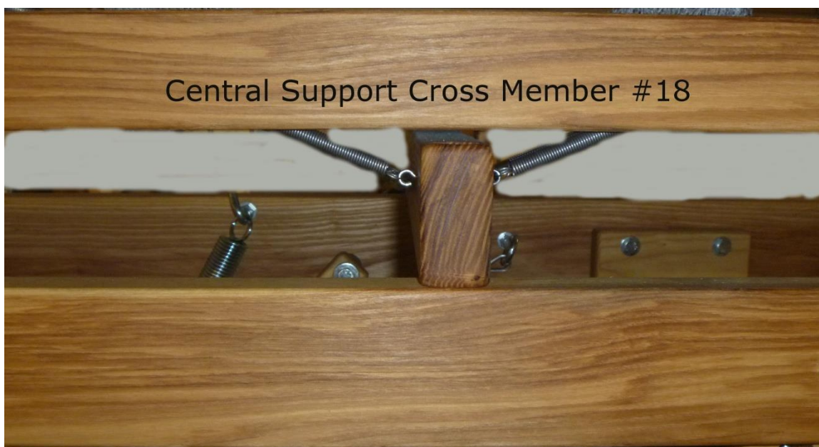
Figure 22 - Support central Cross Member
