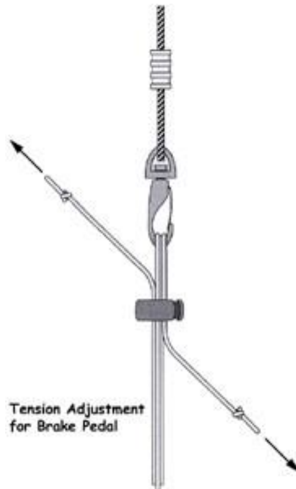
Figure 40 - Tension Adjustment for Brake Pedal
