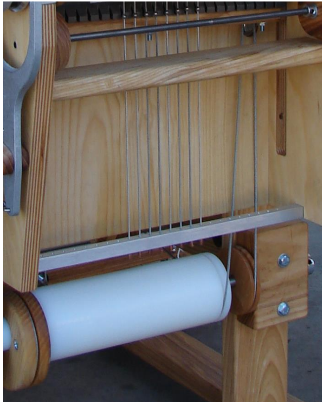
Figure 45 - Cylinder to Dobby Arm Cable
