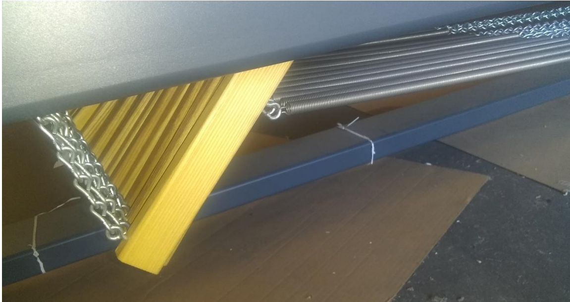
Figure 20 - Harness springs attached to lever
