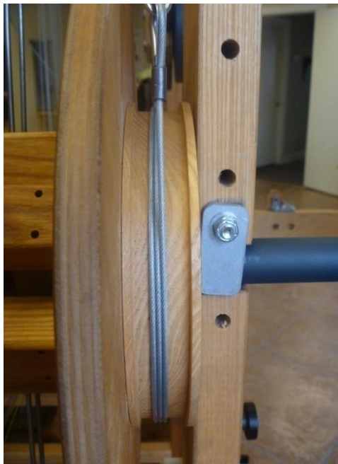
Figure 58 - Tension Cable around Brake Drum
