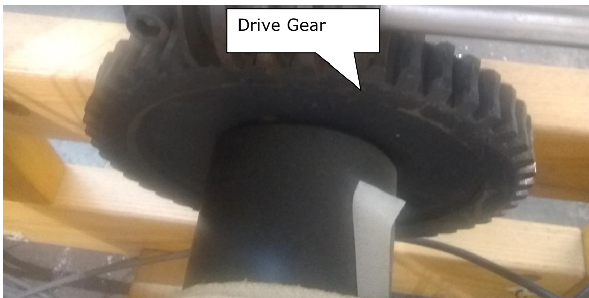
Figure 47 - Gear on cloth storage beam
