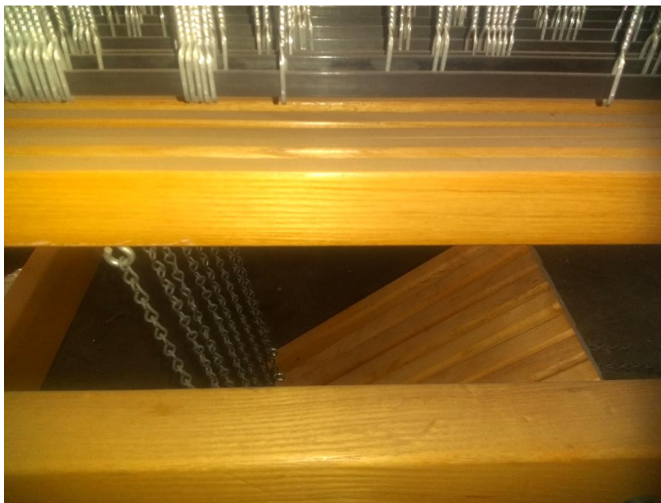
Figure 18 - Spring lever connected to harness
