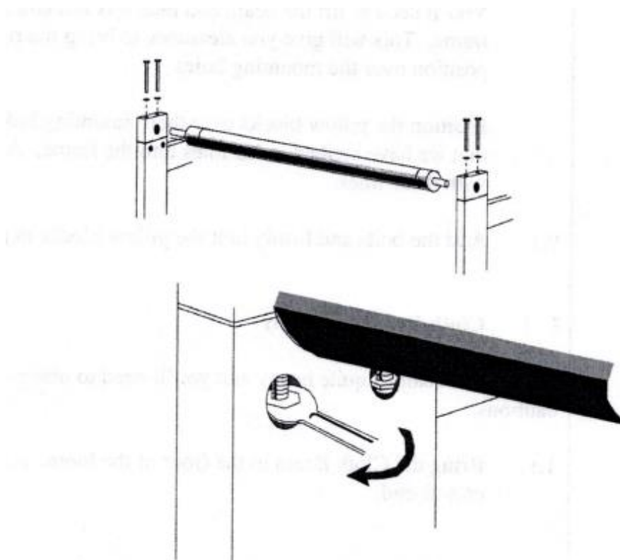
Figure 25 - Installing Cloth Beam
