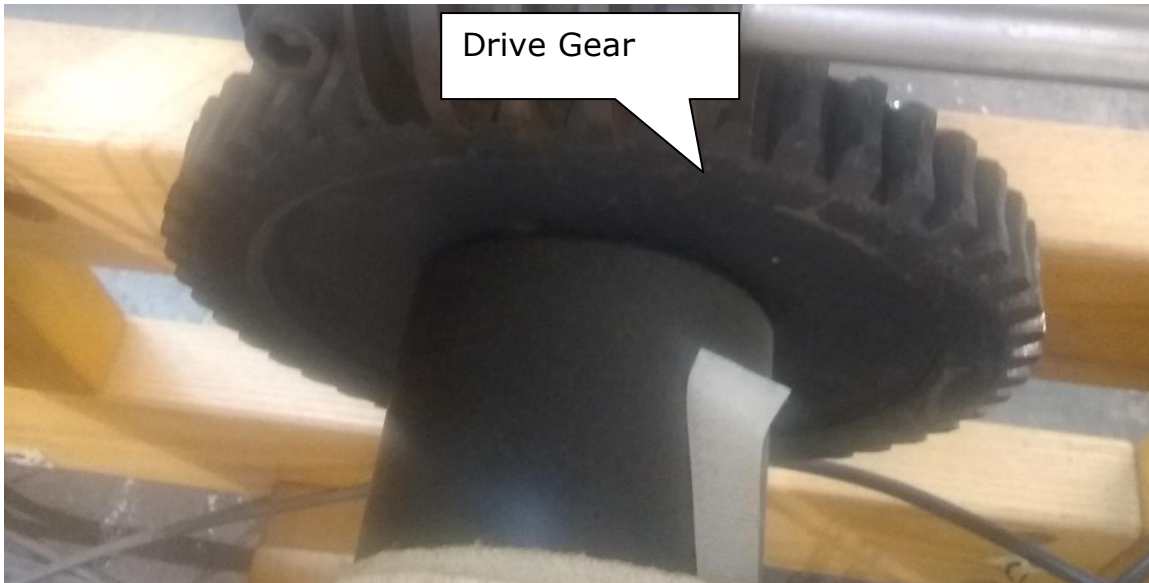
Figure 21 - Gear on cloth storage beam
