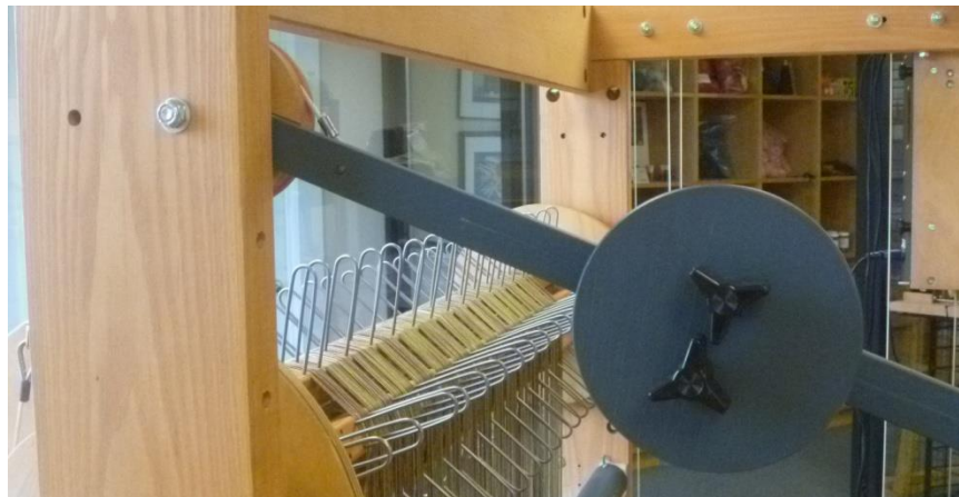
Figure 61 - Tension Arm with Weight
