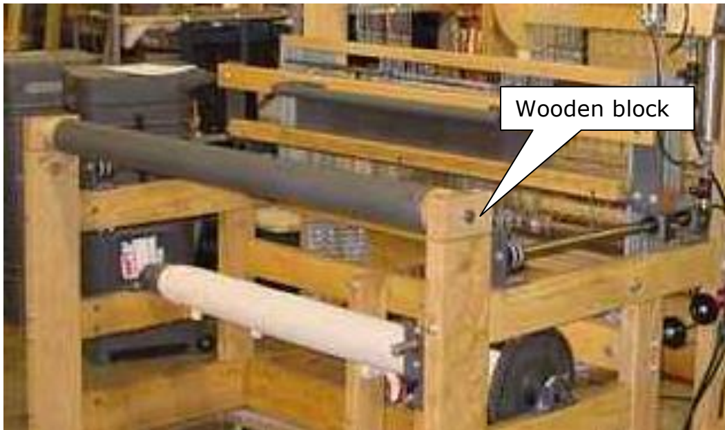
Figure 26 - Cloth beam on wooden frame
