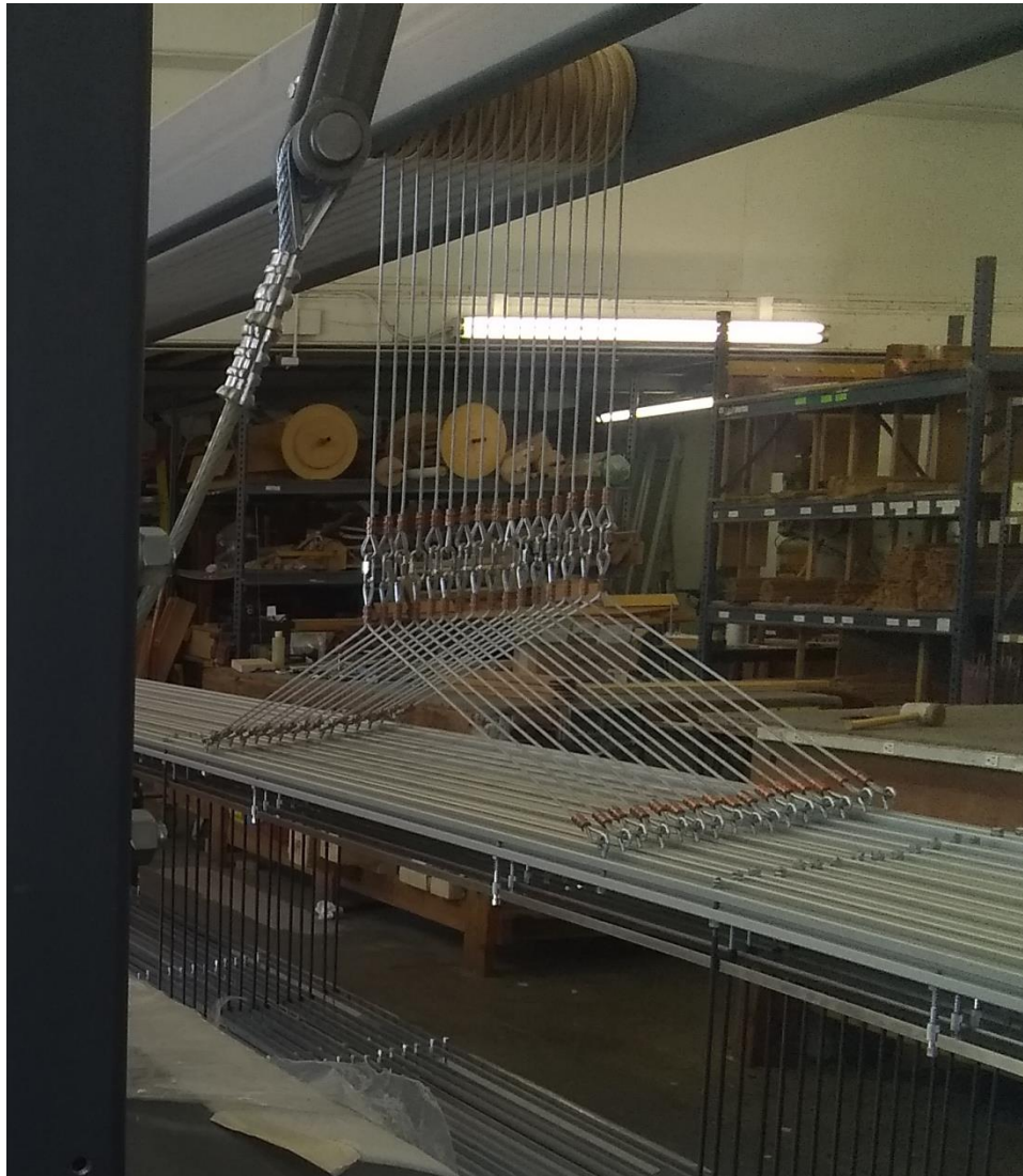
Figure 16 - Harness cables on longer loom
