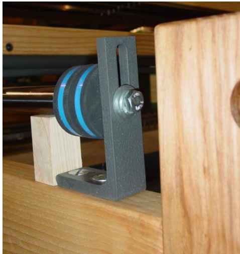
Figure 11 - Adjustment bolt on beater
