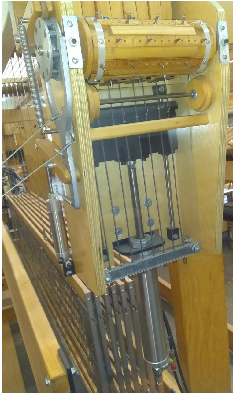
Figure 39 - Air lift on loom
