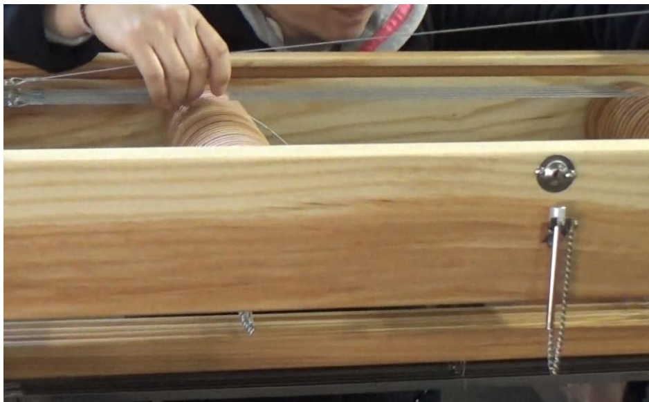
Figure 25 - Placing top harness cables
