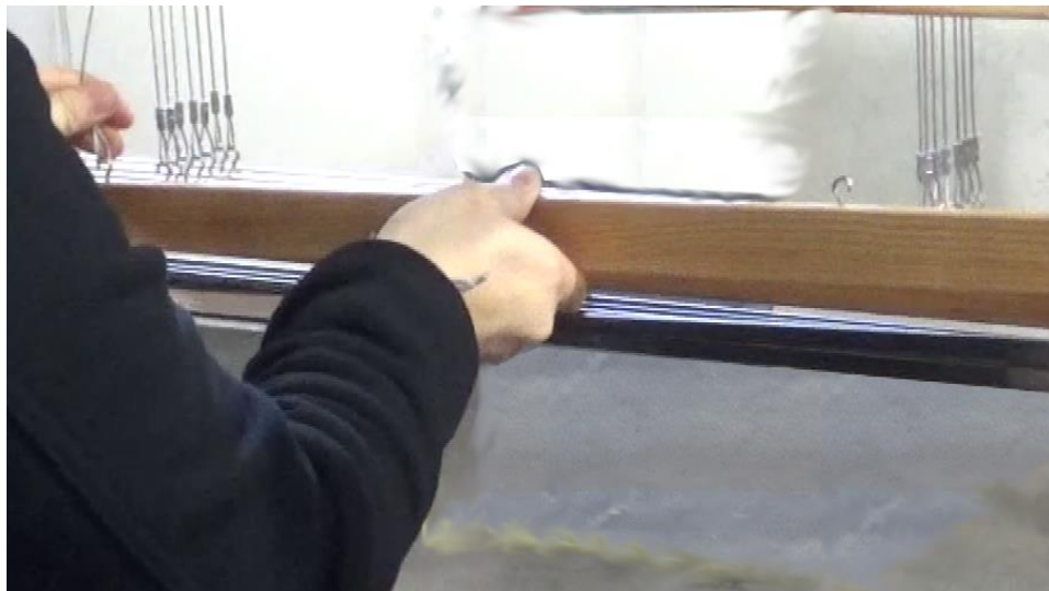
Figure 27 - Hanging harnesses, top cables
