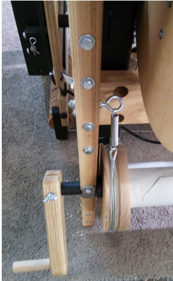
Figure 70 - Tension system for second beam
