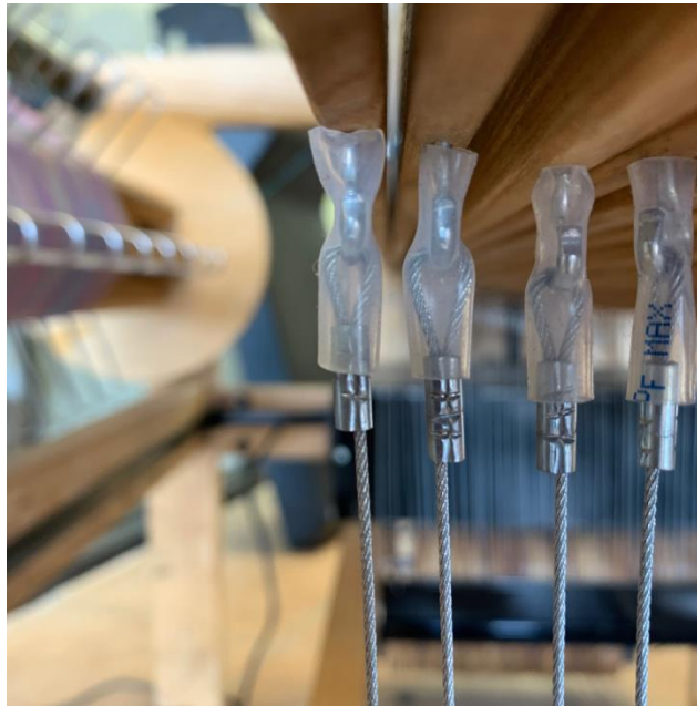
Figure 35 - Bottom harness cables with cable retainers
