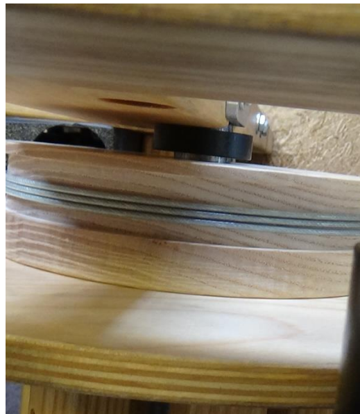
Figure 66 - Warp Beam Spacer on brake side
