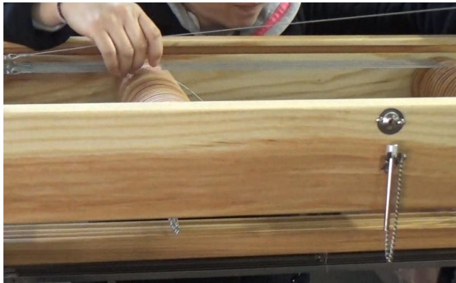
Figure 31 - Placing top harness cables
