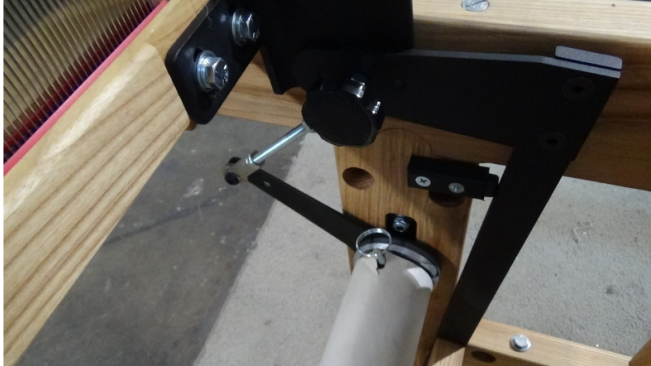
Figure 50 – Beater attached to cloth advance
