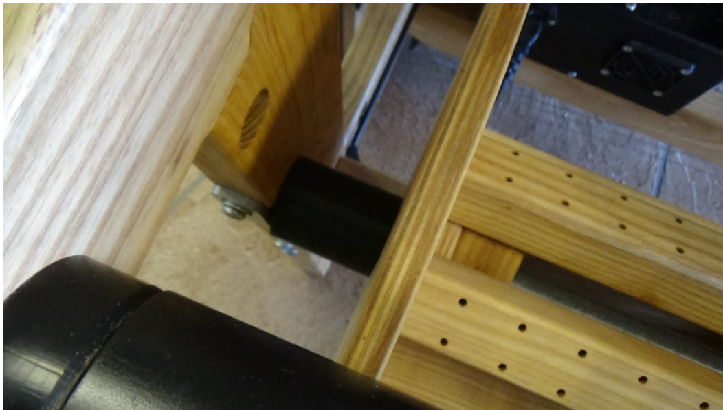
Figure 67 - Warp Beam Spacer on non-brake side
