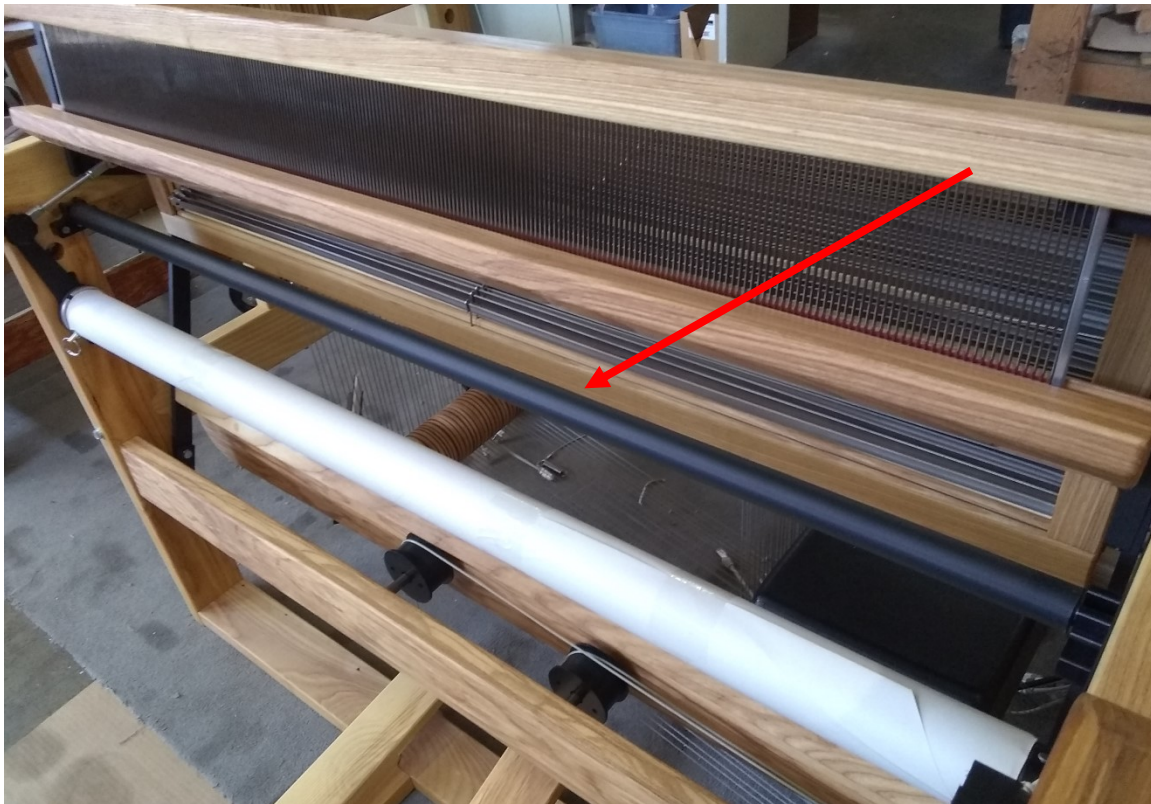
Figure 58 – Cloth guide roller on loom
