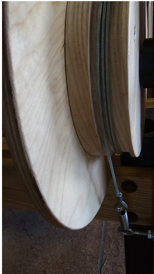
Figure 70 - Tension system from back of loom
