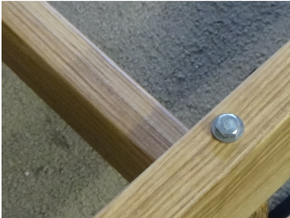
Figure 13 – Bolt for bottom harness pulley support assembly
