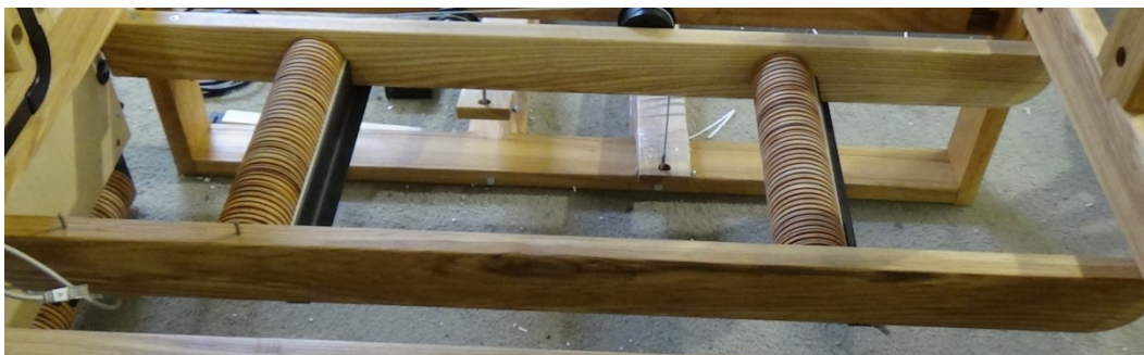
Figure 12 - Bottom Harness Pulley Support Assembly
