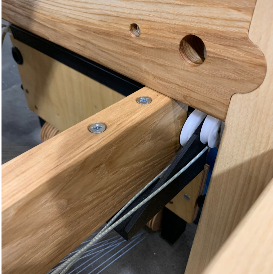
Figure 24 – Lower treadle pulley assembly from inside loom
