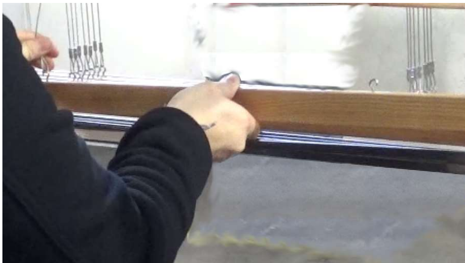
Figure 31 - Hanging harnesses, top cables
