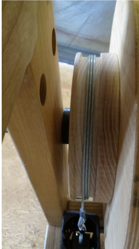
Figure 71 - Tension system from inside loom
