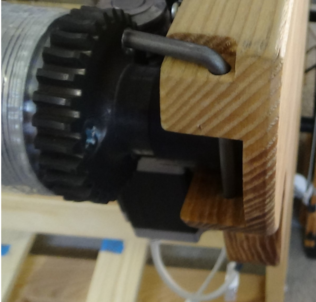
Figure 64 – Retainer pins for cloth beam
