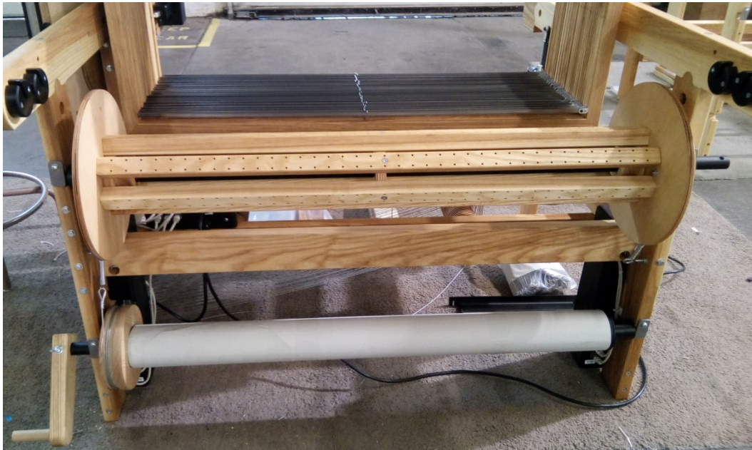
Figure 73 – Loom with two warp beams
