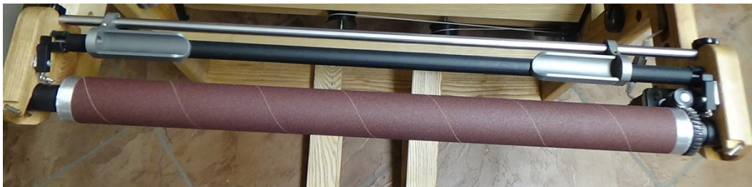
Figure 82 – Ring temple rod on loom
