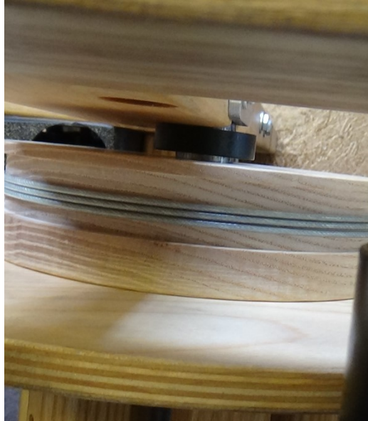
Figure 68 - Warp Beam Spacer on brake side
