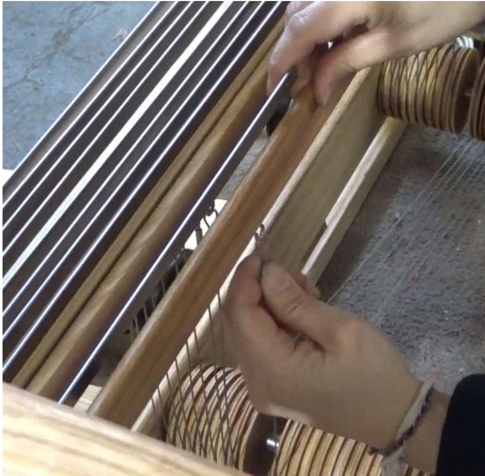
Figure 33 - Hanging harnesses, bottom cables
