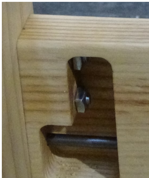
Figure 15 - Front cross member attached to side frame
