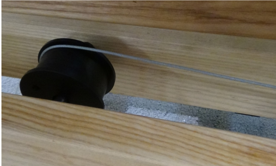
Figure 39 - Left treadle pulley with cable
