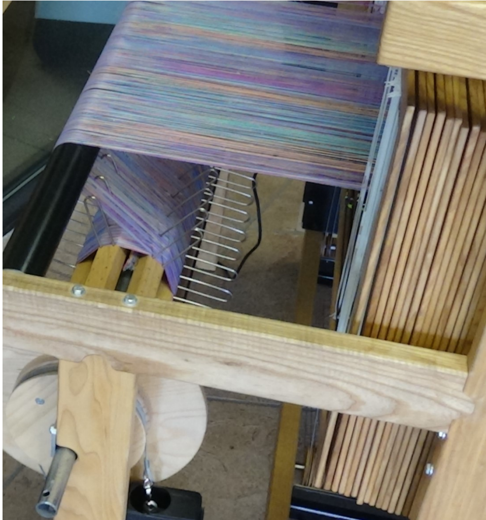
Figure 91 – Warp threads entering the heddles
