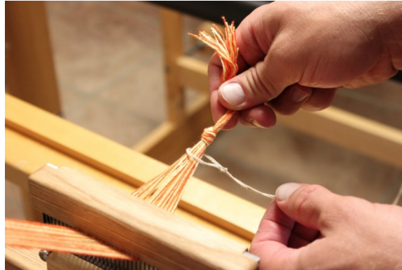
Figure 105 - Place Extension Cord Around Thread Bundle
