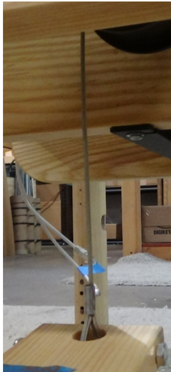
Figure 40 - Left treadle cable on treadle
