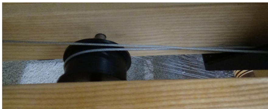
Figure 41 - Right treadle pulley with cable
