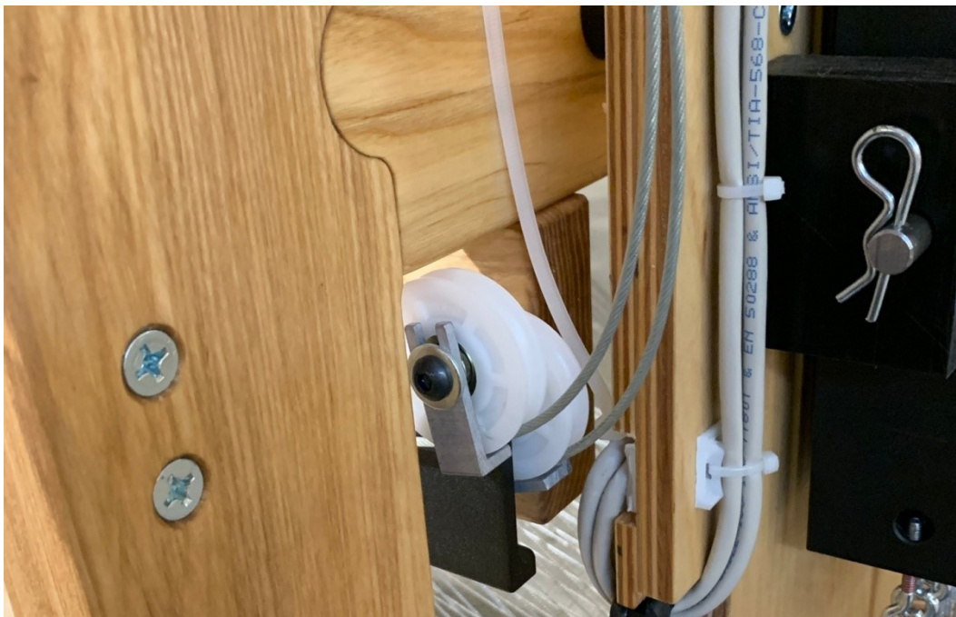
Figure 23 – Lower treadle pulley assembly
