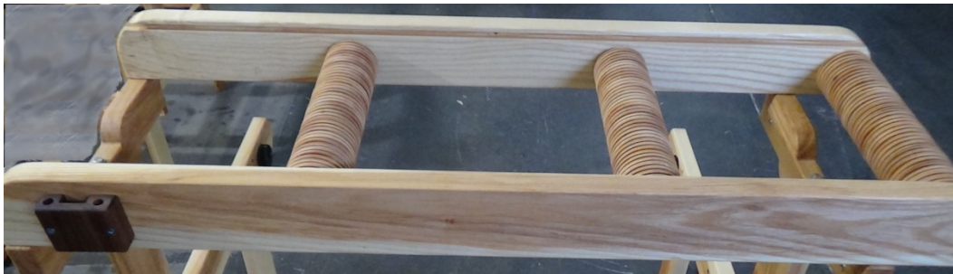
Figure 20 - Top Harness Pulley Support Assembly
