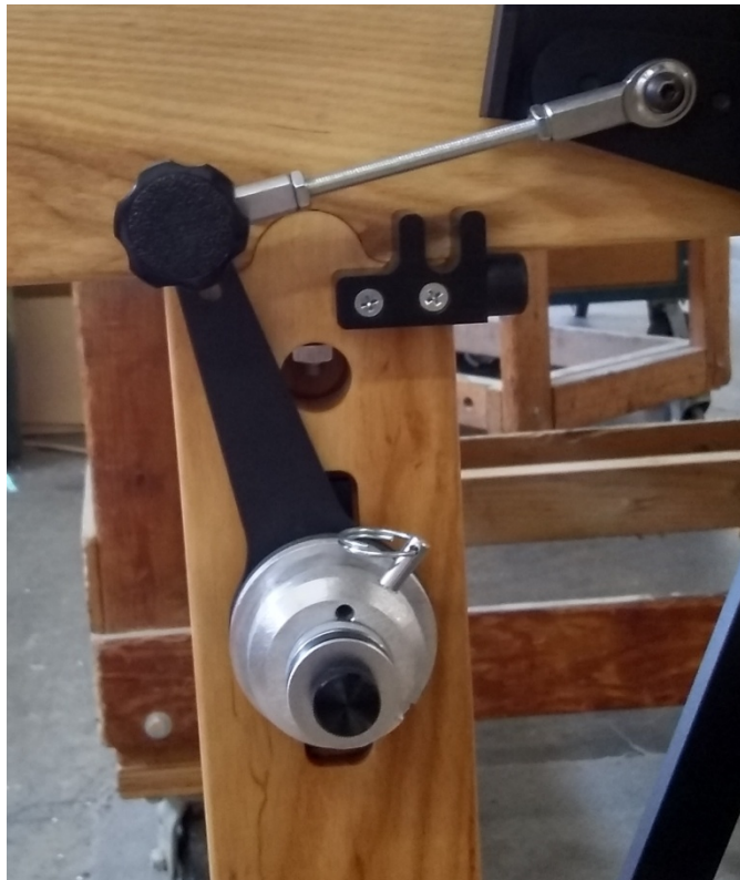
Figure 45 - Cloth Storage Bearing
