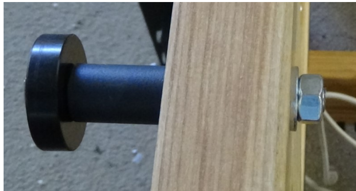
Figure 85 – Track and Mount support with bolt
