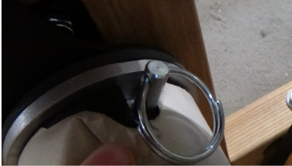
Figure 46 - Cloth Storage Beam Pin
