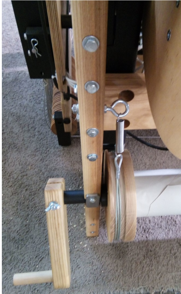
Figure 72 - Tension system for second beam
