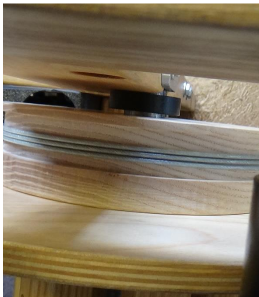
Figure 67 - Warp Beam Spacer on brake side
