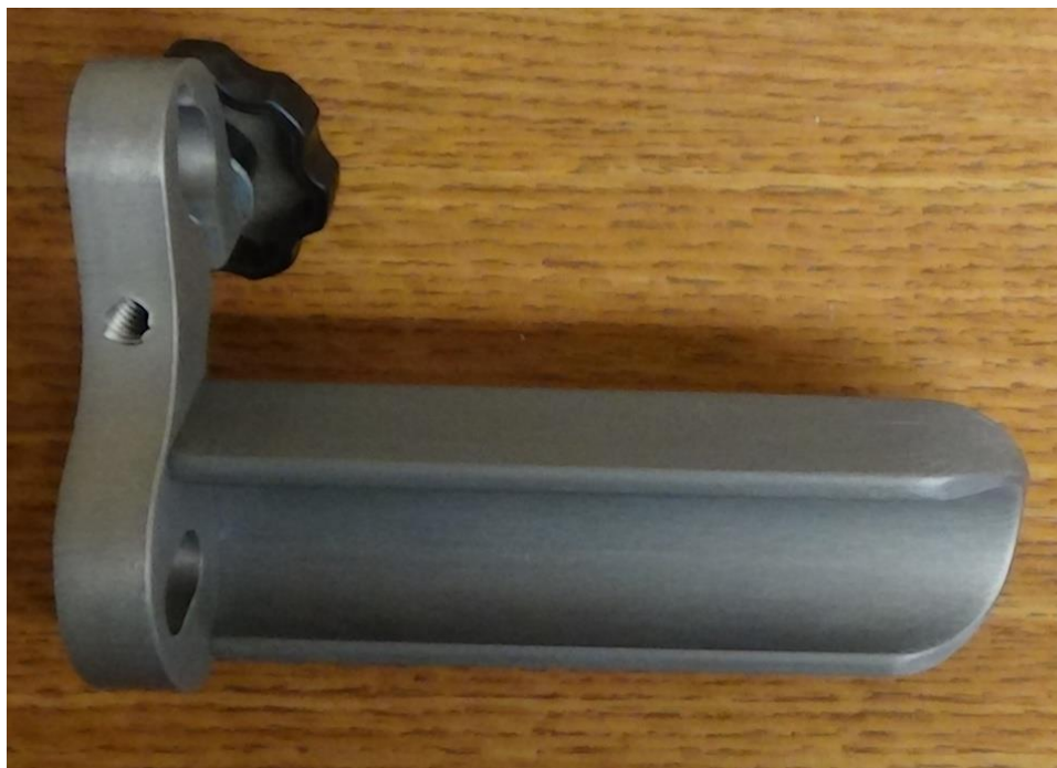
Figure 78 – Ring temple support with knob
