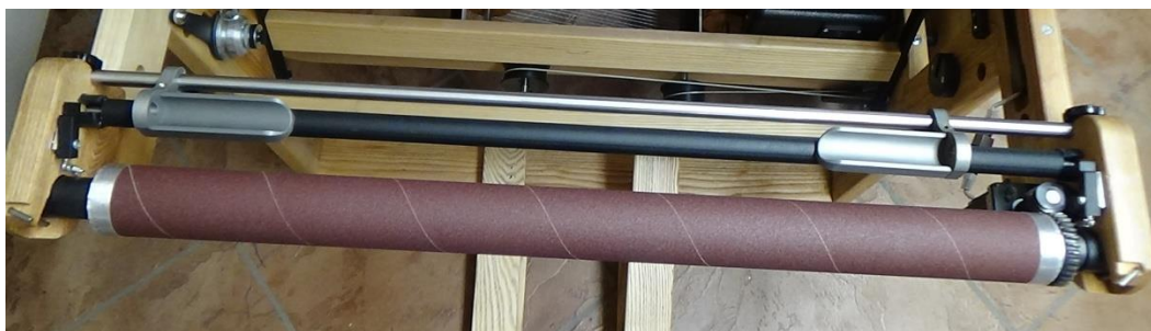
Figure 81 – Ring temple rod on loom
