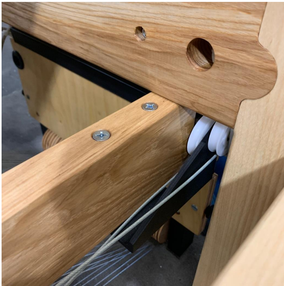
Figure 24 – Lower treadle pulley assembly from inside loom
