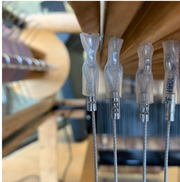
Figure 33 - Bottom harness cables with cable retainers
