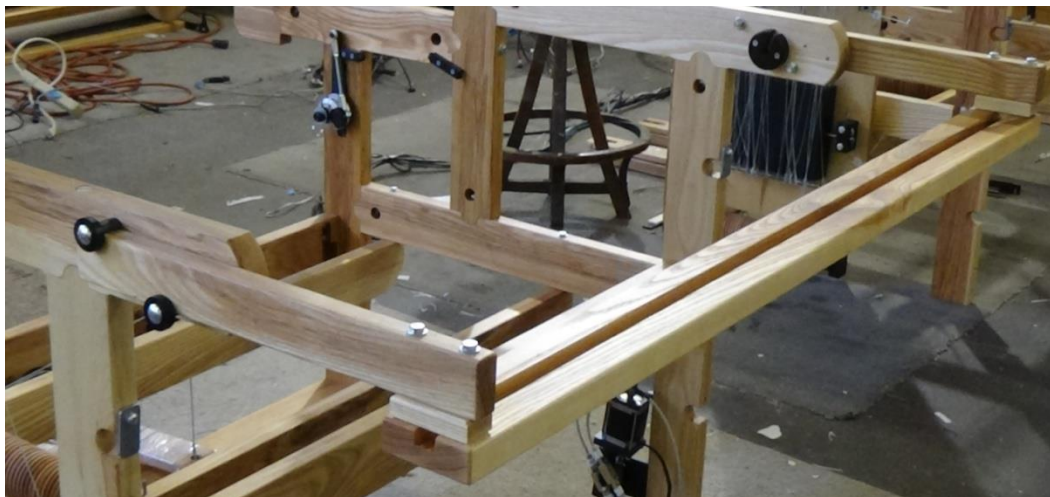
Figure 86 - Attach Track & Mount Arms
