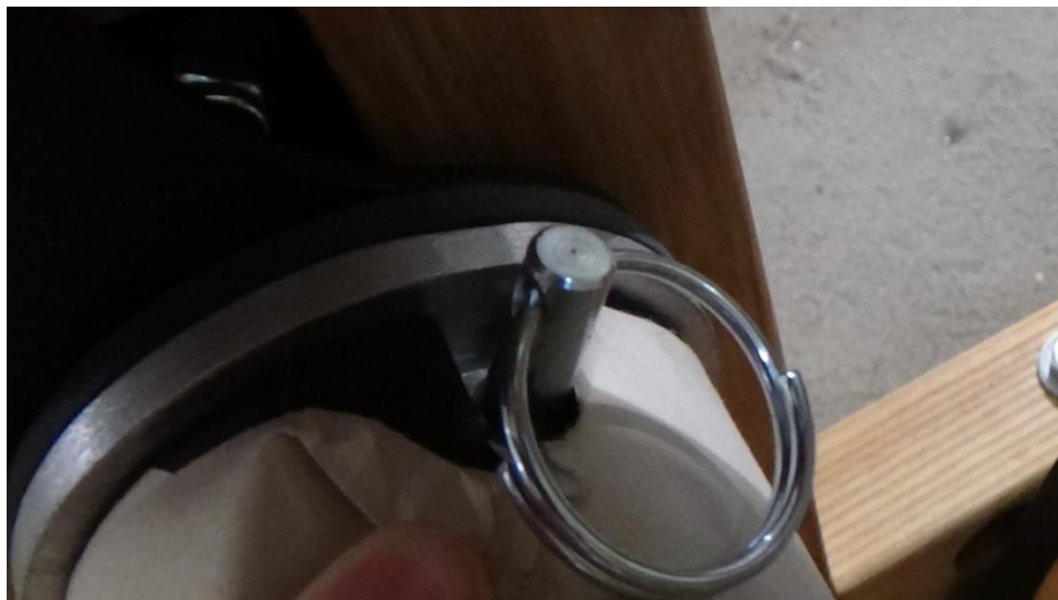
Figure 46 - Cloth Storage Beam Pin
