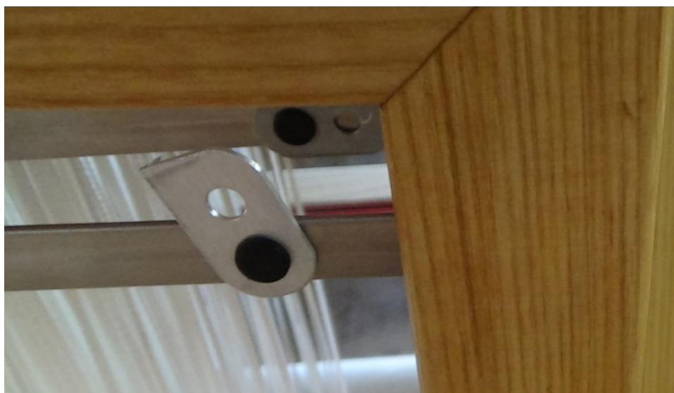
Figure 35 - Keeper on harness opened from back
