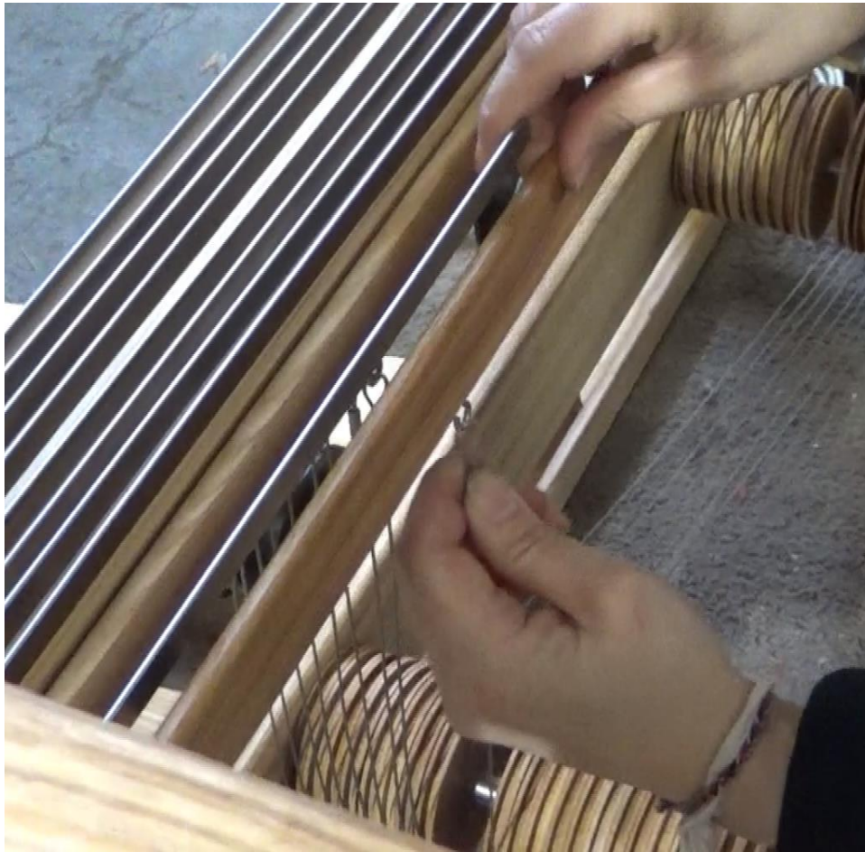
Figure 32 - Hanging harnesses, bottom cables
