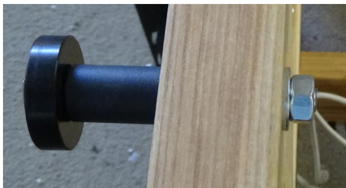
Figure 84 – Track and Mount support with bolt
