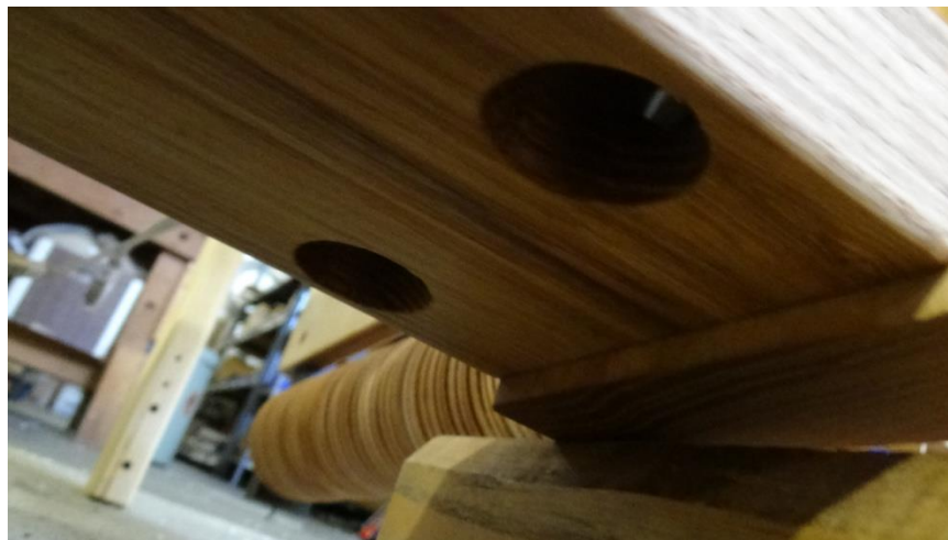
Figure 18 – Closeup of nut access holes
