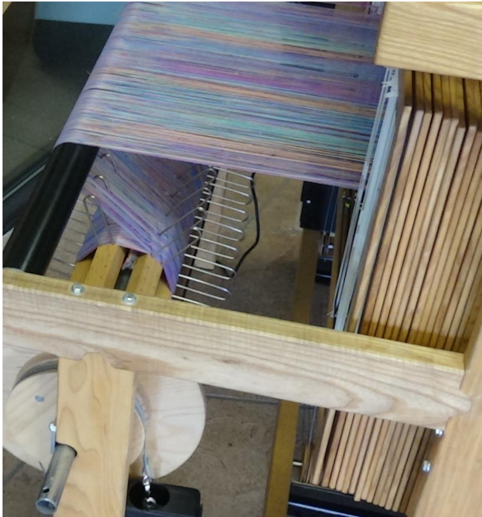
Figure 85 – Warp threads entering the heddles
