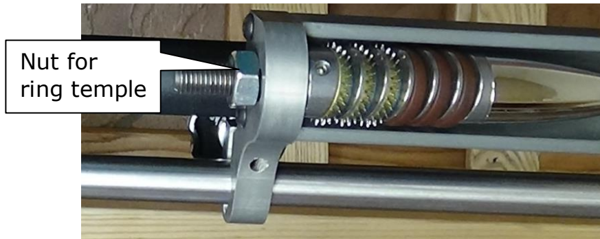
Figure 77 – Ring temple on loom
