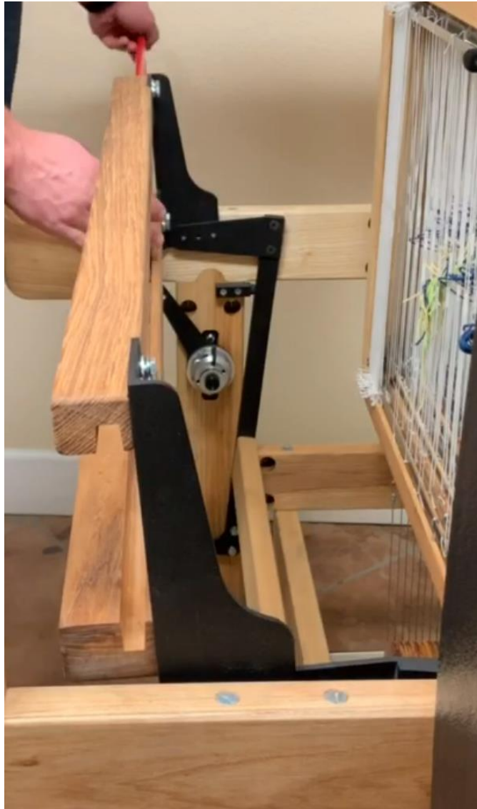
Figure 105 – Push the reed out
