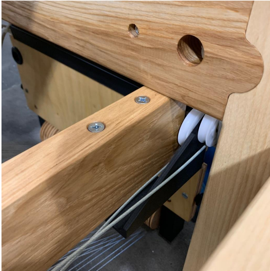
Figure 24 – Lower treadle pulley assembly from inside loom
