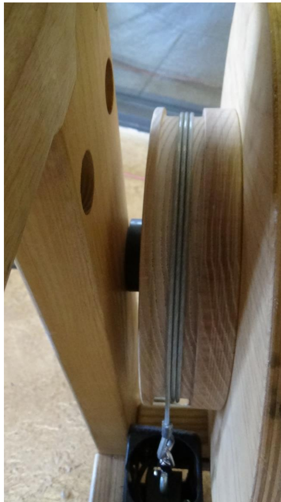
Figure 65 - Tension system from inside loom
