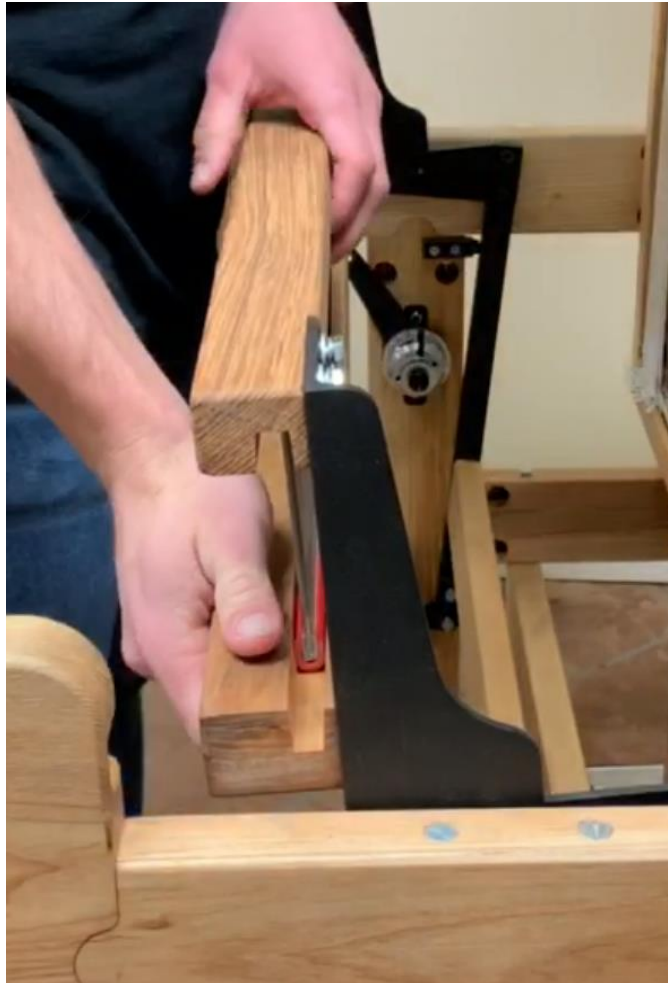
Figure 104 – Push down bottom support
