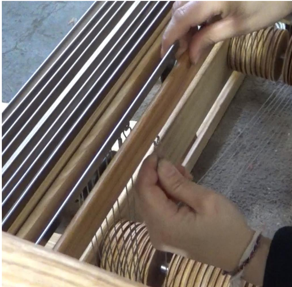
Figure 29 - Hanging harnesses, bottom cables
