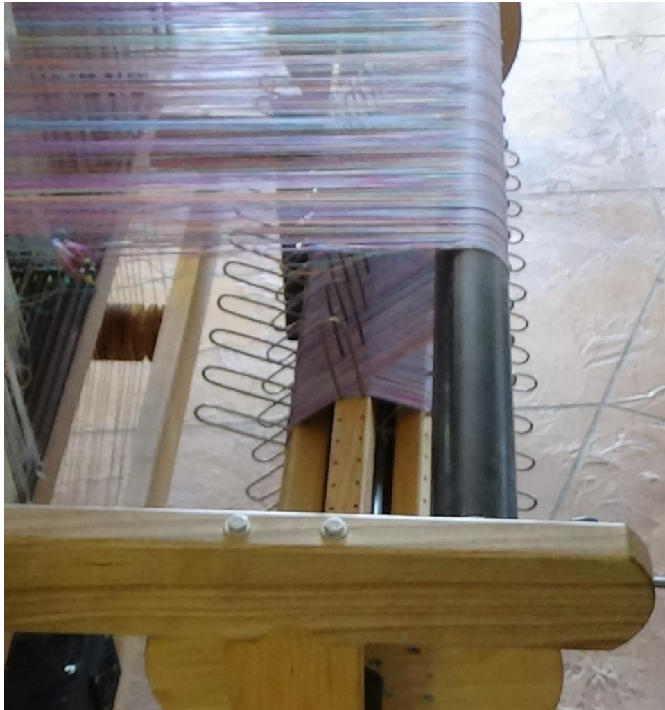
Figure 84 – Warped beam from back
