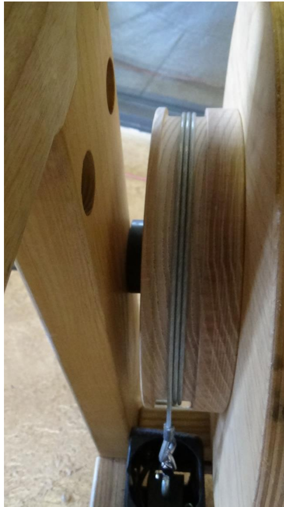
Figure 71 - Tension system from inside loom
