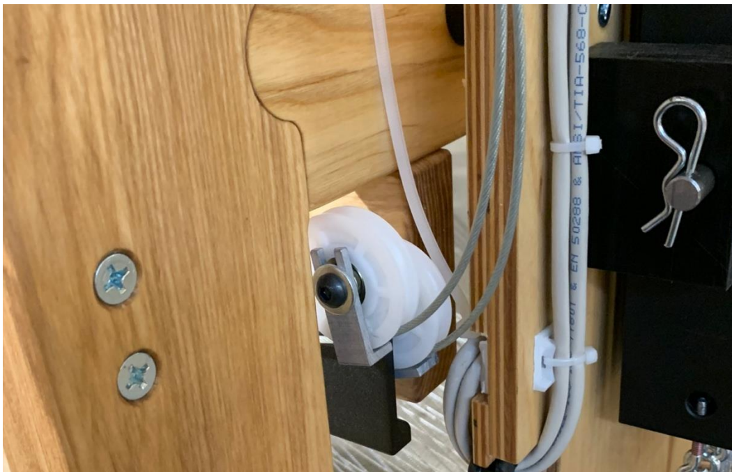
Figure 23 – Lower treadle pulley assembly
