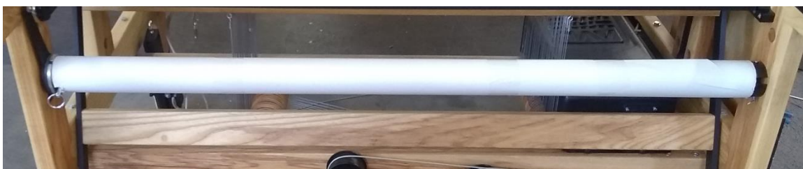
Figure 47 - Cloth Storage Beam
