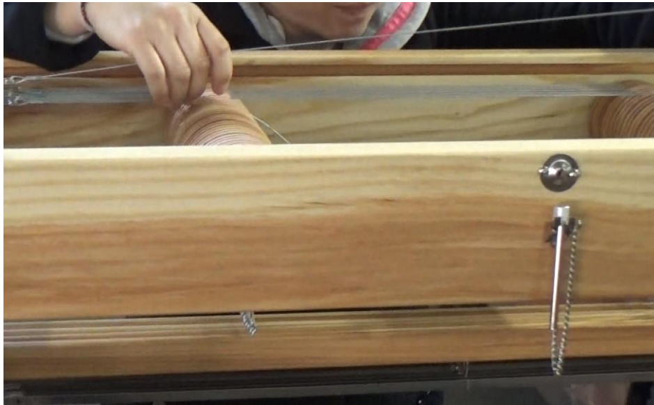
Figure 29 - Placing top harness cables
