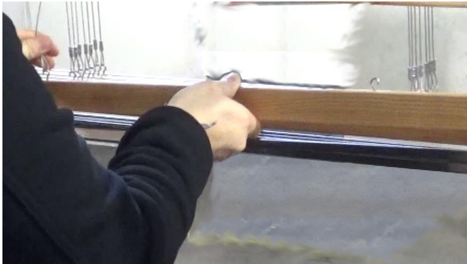
Figure 31 - Hanging harnesses, top cables
