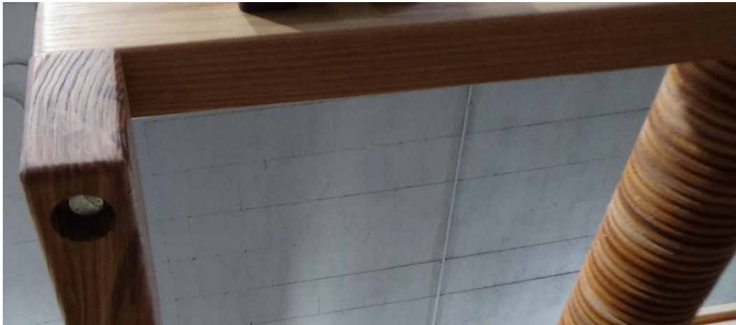
Figure 21 – Bolt for top harness pulley support assembly
