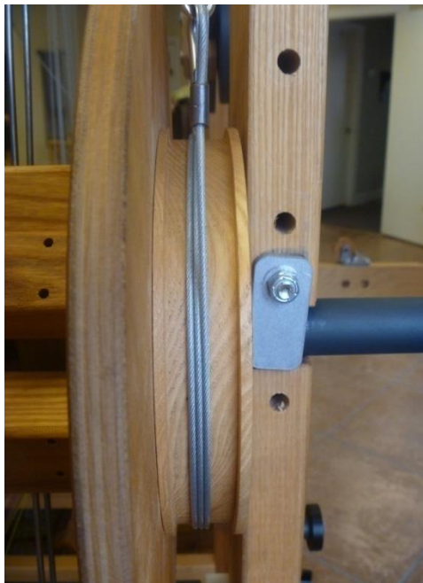
Figure 34 - Tension Cable around Brake Drum
