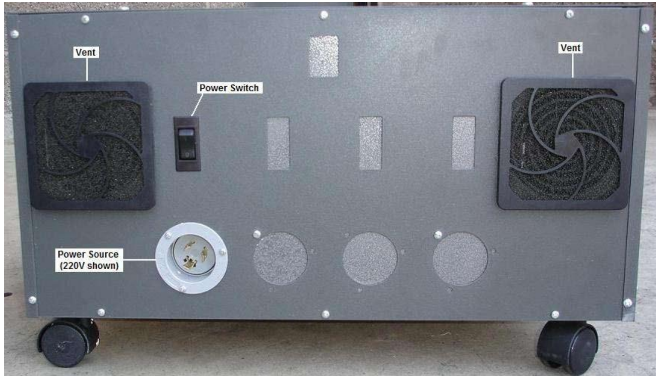
Figure 92 - Control Box, Side 1 (Showing Vents, Power Switch and Power Source)
