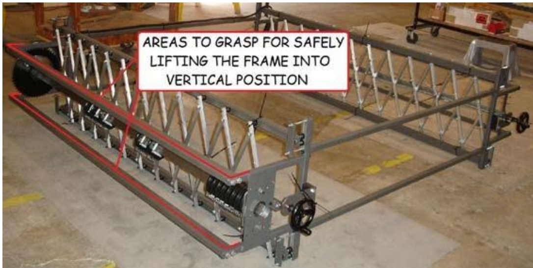
Figure 22 - Areas for grasping the Module Frame during the lift
