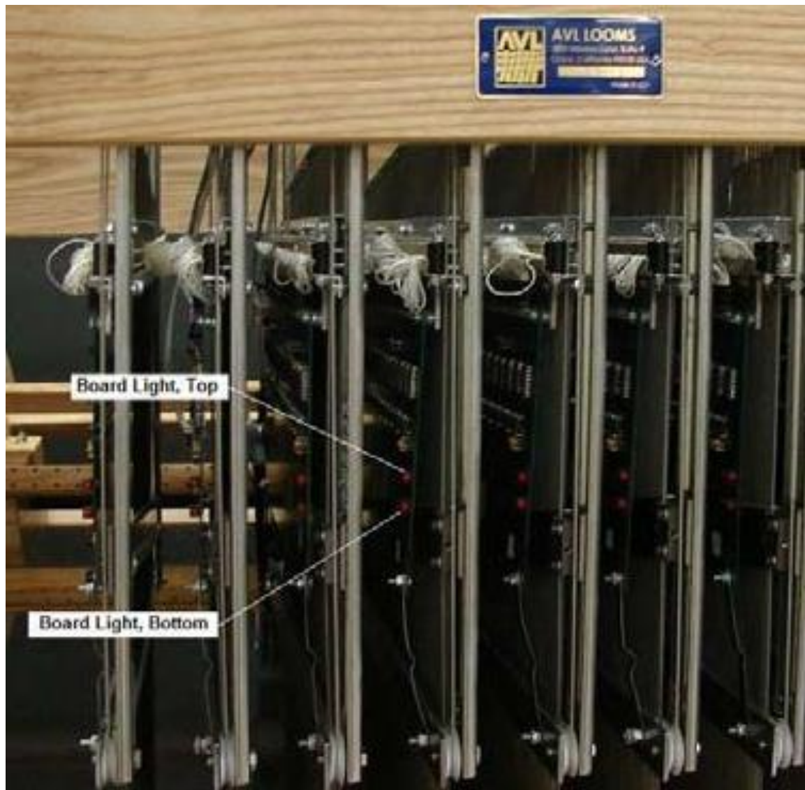
Figure 104 – Modules, front view showing board lights
