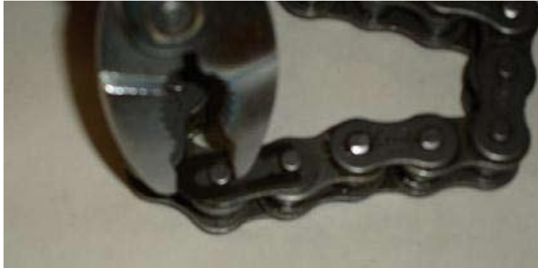
Figure 86 - Closing the Connecting Link Clip with Pliers
