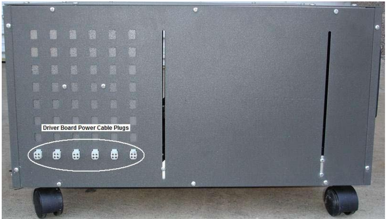
Figure 94 - Control Box Side 3 (Showing Driver Board Power Cable Plugs)
