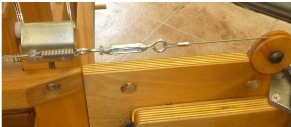
**Figure 78 - Tendeur Flyshuttle**
