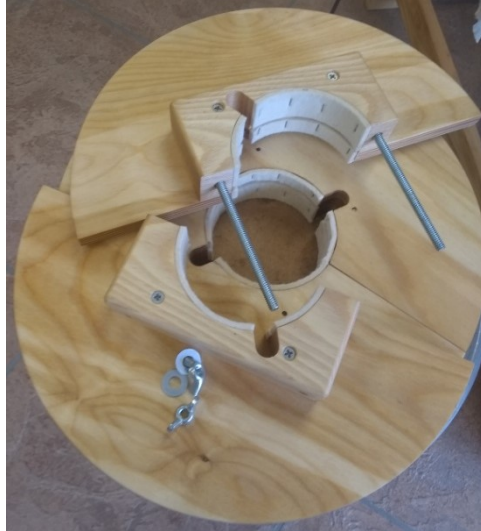
Figure 2 - Warp Beam Flange Halves
