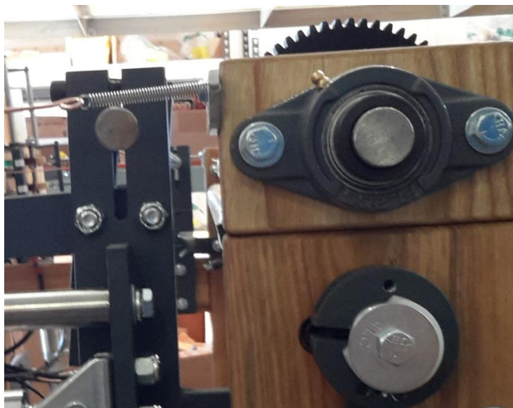
Figure 8 - Fafnir VCJT1 Bearing
