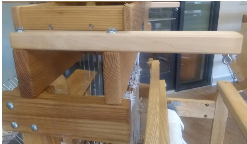
Figure 34 - Flystring support on loom
