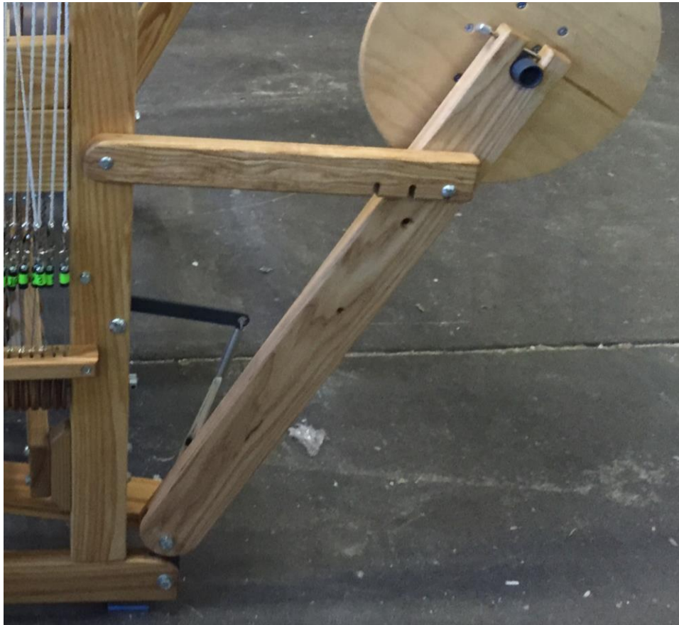
Figure 23 - Support arms for folding legs
