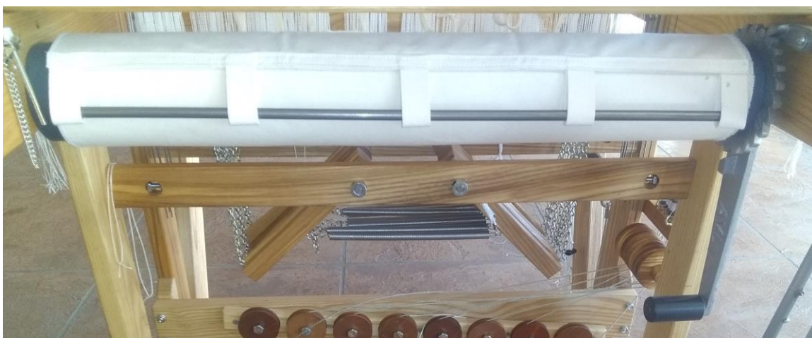
Figure 6 - Cloth Storage Beam
