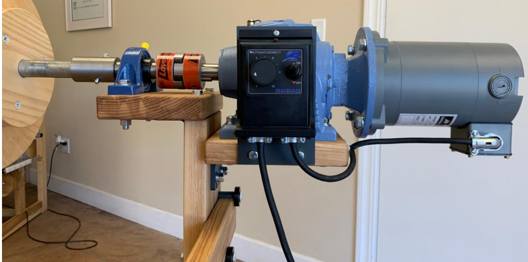
Figure 4 - Motor on Free-standing beam winder
