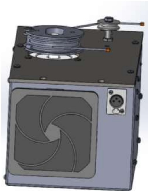
Fig. 2c – E-Lift Cable Routing (front view)
