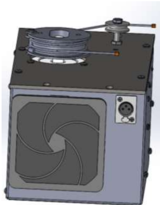
Fig. 2c – E-Lift Cable Routing (front view)
