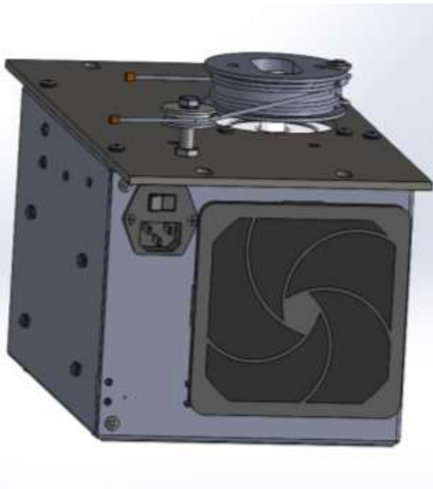
Fig. 2b – E-Lift Cable Routing (rear view)
