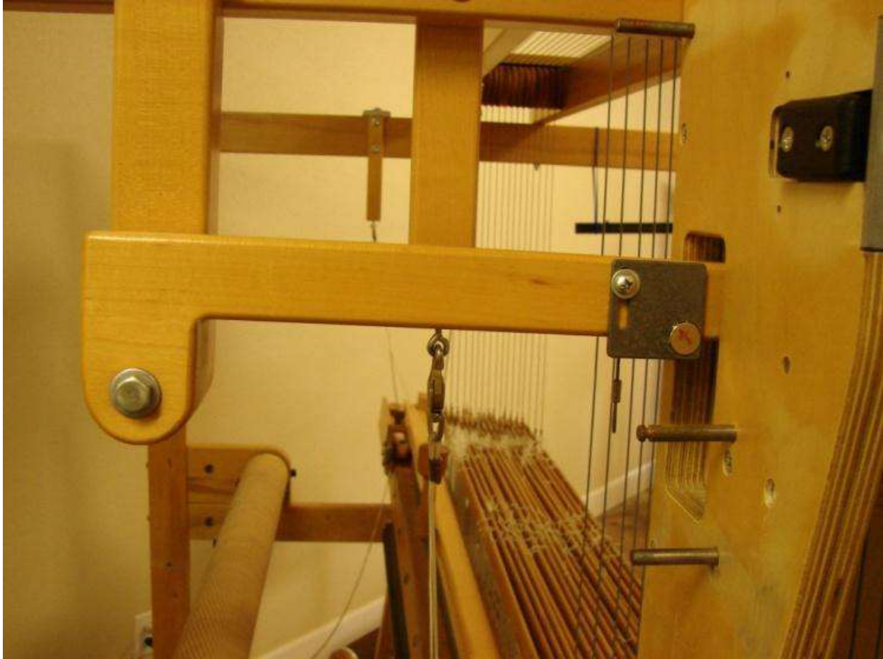
Figure 5 - Magnet Assembly Mounted on Dobby Arm
