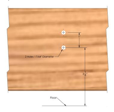
2) Drill thru the frame at the marked holes using a size H (.266") diameter bit.
