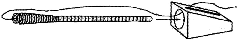
Figure 34 - Bobbin Winding Guide
