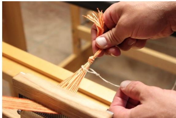
Figure 20 - Place Extension Cord Around Thread Bundle
