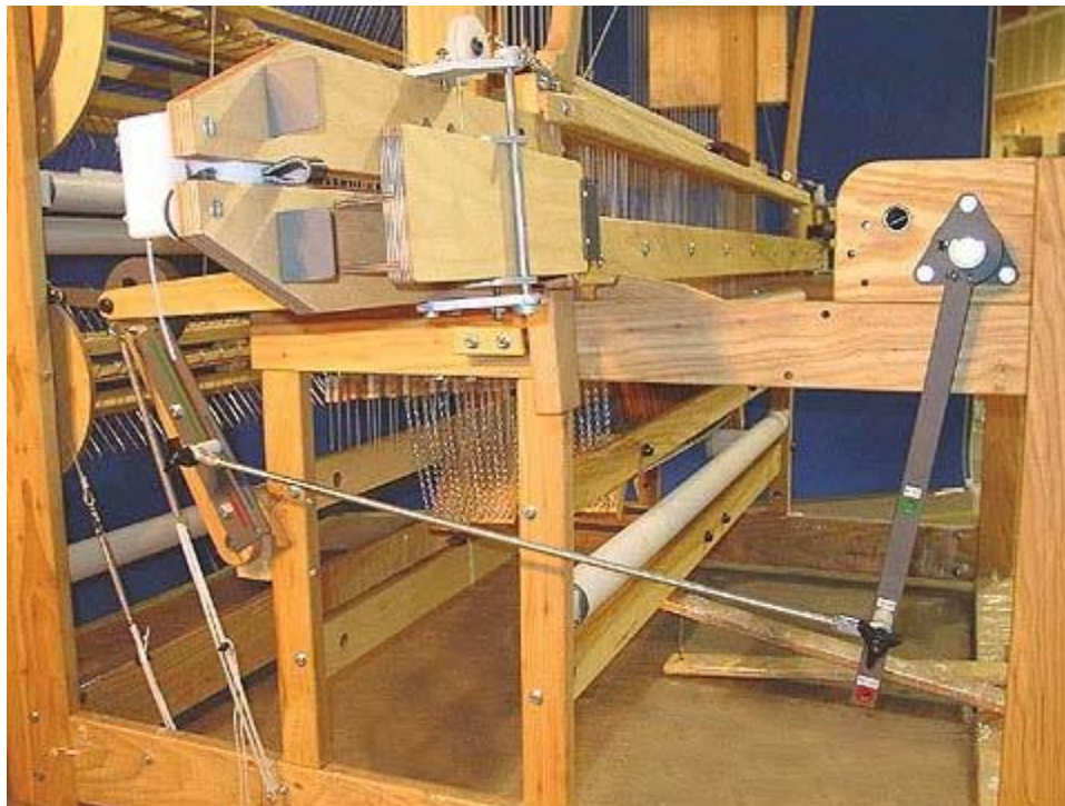
Figure 36 - Overhead Beater with Automatic Advance
