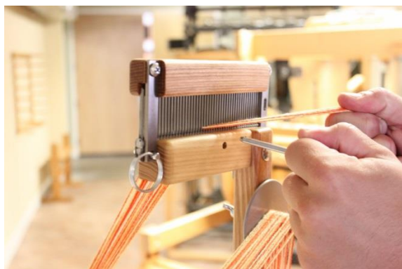
Figure 18 - Remove Raddle from Top Position
