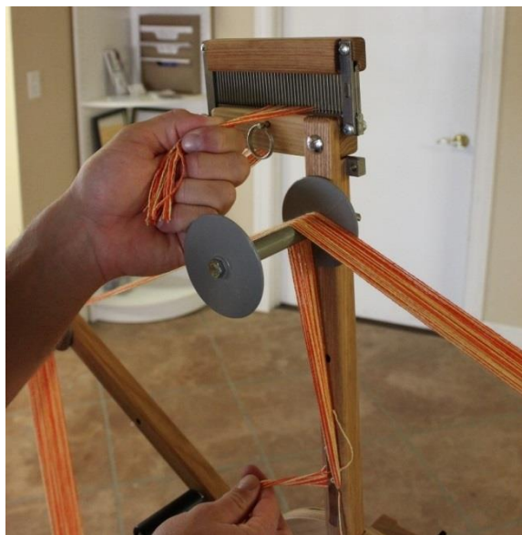
Figure 17 - Hold Threads at Raddle
