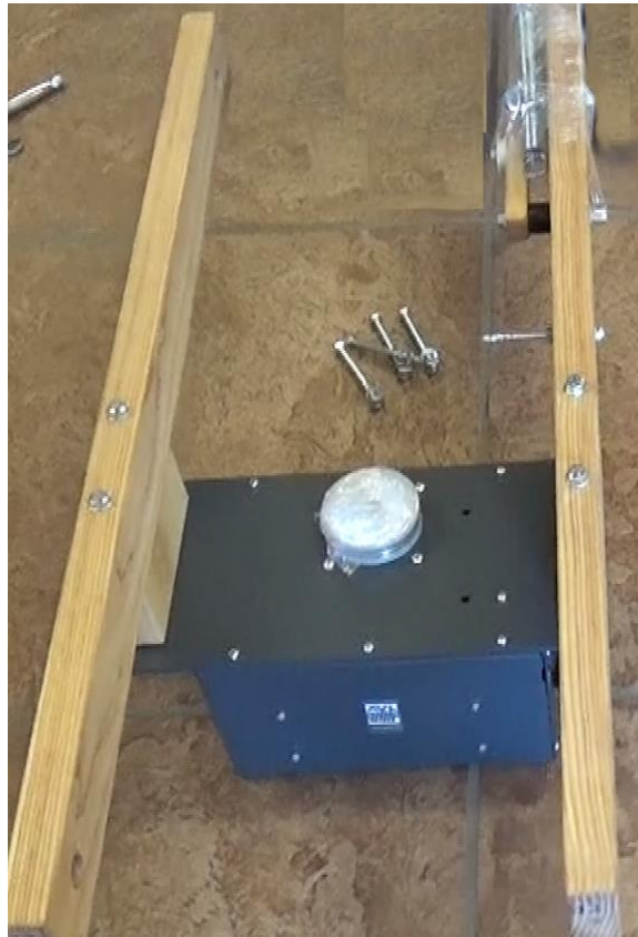
Figure 30 - E-lift attaché aux supports
