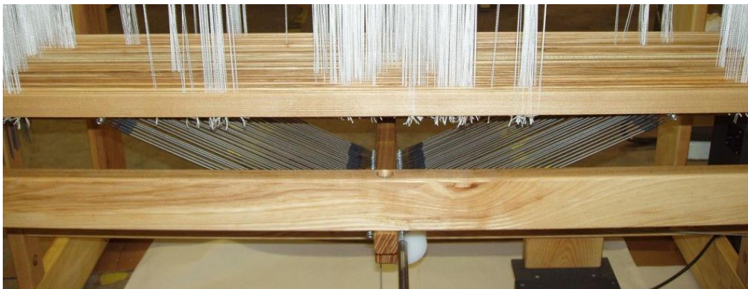
Figure 34 - 32/40 Harness Spring System
