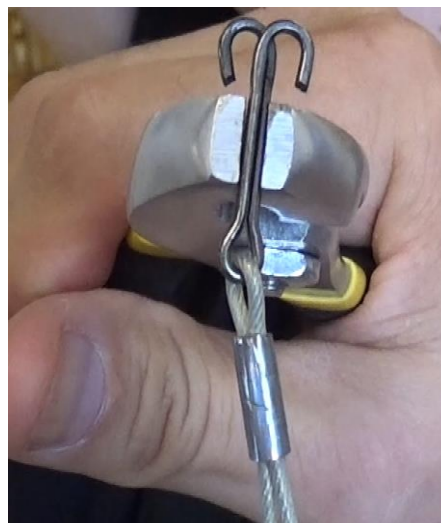
Figure 54 - Clip opened with pliers
