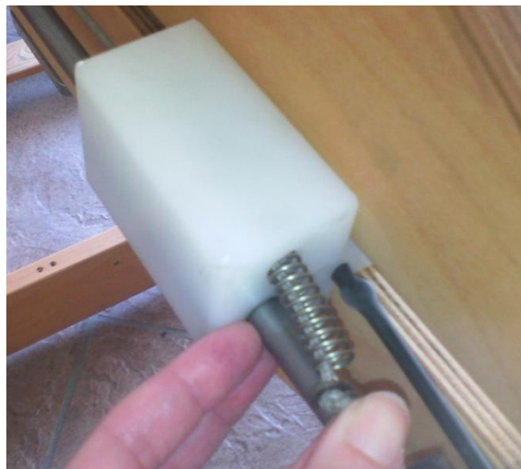
Figure 114 - Spring and washer on Flyshuttle cord
