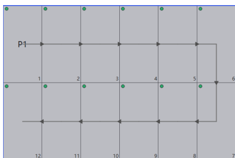
Figure 4-10 Cabinets connected automatically
