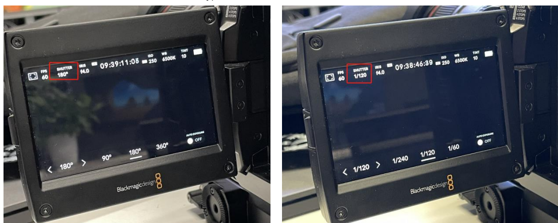
Figure 2-14 Camera shutter angle/speed example (the position of parameters may vary among different camera models, for reference only)
