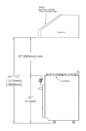
The bottom of the hood should be 35" min. to 36" above the counter top. This would typically result in the bottom of the hood being 66" to 72" above the floor. These dimensions provide safe and efficient operation of the hood.
