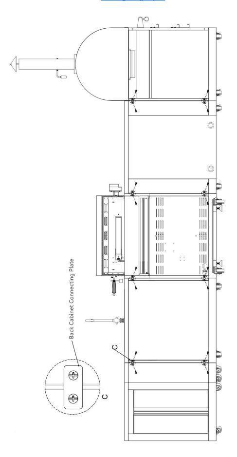
You Thor Kitchen Outdoor Cabinet could be connected with any other Thor Kitchen Our Door Cabinet models. For Back Panel Connections, use Back Cabinet connecting plate with 2 pcs % screws (Part # 06.02.00093-000-A0) to connect both Cabinets.
