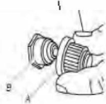
A. Igniter push button B. "AA" size battery
