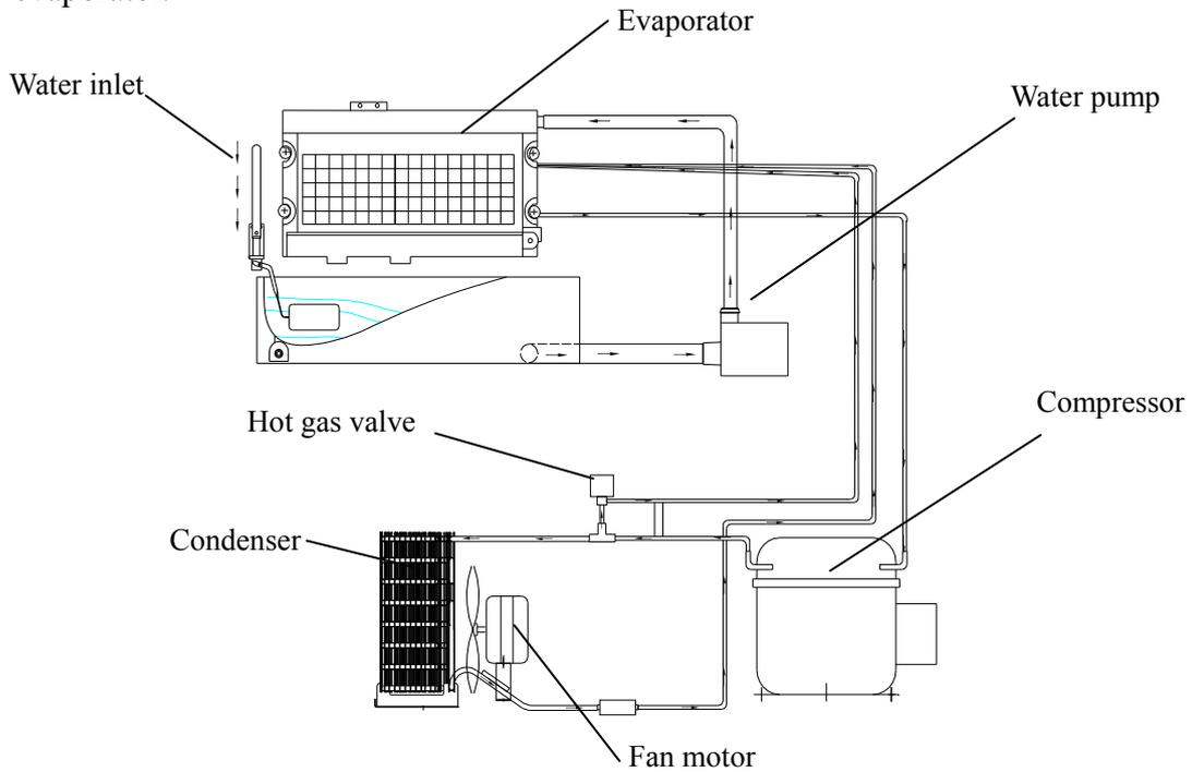
***How the pump out water drain system operates***
