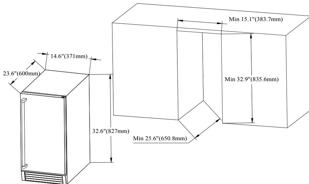
When installing the ice maker under a counter, follow the recommended spacing dimensions shown. Allow at least 2" (50.8 mm) of clearance at rear, and ¼" (6.35mm) at sides for proper air circulation.
