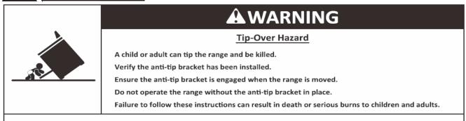
Show specific manufacturer illustrations for checking installation/engagement of anti-tip brackets.
