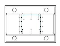
6.Slide the upper chimney onto the support frames
