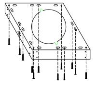
3.Attach the angle bars to the ceiling mount using (16) M5 screws. (if your Island hood is going to be used in ducted mode, connect the ducting hose to the ceiling mount at this point.)
