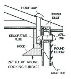
Flexible ductwork is not recommended. Flexible ductwork creates back pressure and air turbulence that greatly reduces performance. USE ONLY METAL DUCTWORK. Make sure there is proper clearance within the wall or floor for exhaust duct before making cutouts. Do not cut a joist or stud unless absolutely necessary. If a joist or stud must
