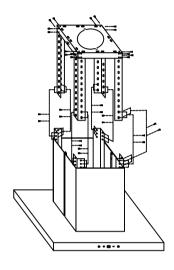
8.Fix the upper chimney to the ceiling mount using (2) M4 screws
