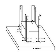
5.Slide the lower chimney onto the support frames connect the main body to the lower chimney by (6) M4 screws from the bottom of the hood
