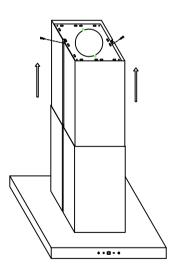
9.If you are going to using the hood in extraction moude (ducted) ,you should attach the ducting hose to the ceiling.
