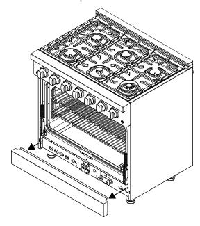
5. Remove the kick plate by unscrewing 3 screws securing it to the oven — 2 on each side of the top lip and 1 in the middle, as shown above. Then, lift up and pull out of the holes on each side to remove the kick plate. To install a new kick plate, position the kick plate into the holes on each side of the range and then replace the same 3 screws.
