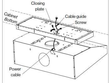
4) Place the hood under the non-duct flue kit and slide the hood into position so the wing of the bracket mounted on the top of the hood is aligned with the mounting brackets supplied.
