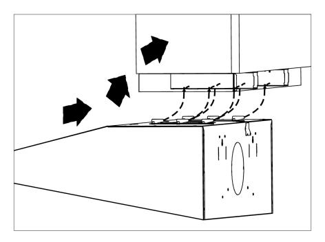
5) Lock the hood with (2) M4 x 10 mm Safety Screws.
