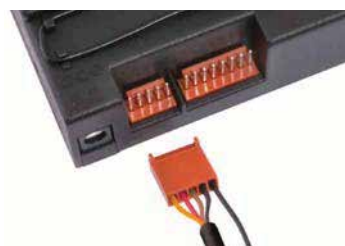
Image 3: Insert plug connector into the receiver.
