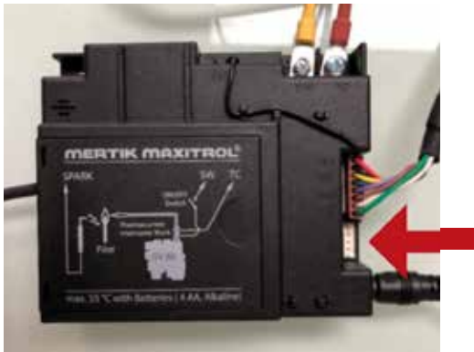
Image 1: Location of wall switch harness connection indicated by arrow
