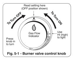
For your convenience and safety; when the control knob is turned to the ON position, the gas flow indicator will change from blue to red. (Red indicates gas flow.) See Fig. 5-1.
