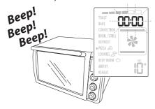
Turn the TOAST COLOR/TIME dial (G) to adjust up to 10 additional minutes, if necessary, and press the START/STOP button (H) at the end of time, the control will turn off the oven.
