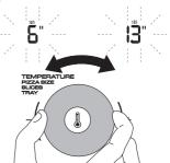
Set the desired level of crusting by turning the TOAST COLOR/ TIME dial (G).
