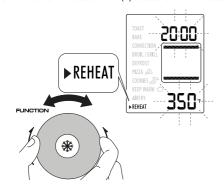
Turn the TEMPERATURE/PIZZA SIZE/SLICES/TRAY dial (M) to set the desired temperature. The default temperature is 350 °F.
