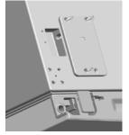
4. Lift up the refrigerator door by 1.97in to remove it.
