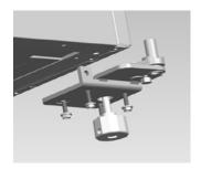
6. Take out the lower left hinge from the accessory bag, and install it on the refrigerator.
