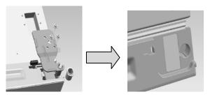
3. Screw off the three bolts fixing the top box cover on the left side, remove the box cover, take the wire harness out of the hole, and transfer the door shaft sleeve from right
